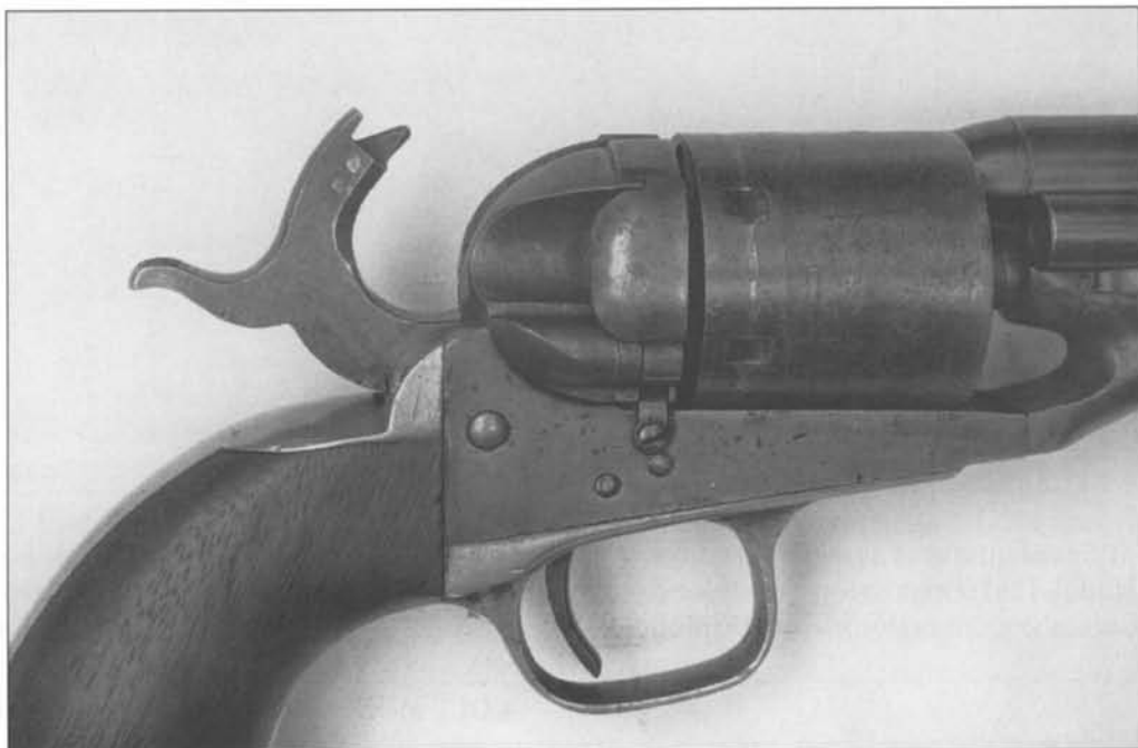
Fig. 6-95 Colt Model 1861 Navy centerfire conversion, serial number 4274, assembly number 34, with external gate spring and blade-type firing pin. (Author's Collection)
