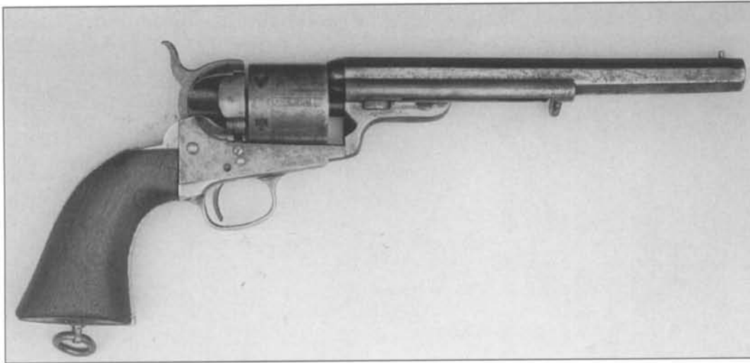
Fig. 6-64 U.S. Navy-Navy Colt Model 1851 early percussion range Richards-Mason conversion with lanyard ring. Serial number 8253. (Author's Collection)
