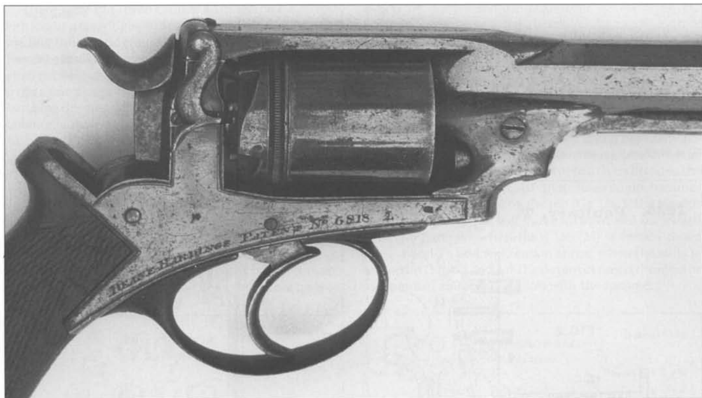
Fig. 4-34 Deane-Harding conversion with firing-pins in each chamber. Serial number 6818. (Author's Collection)
