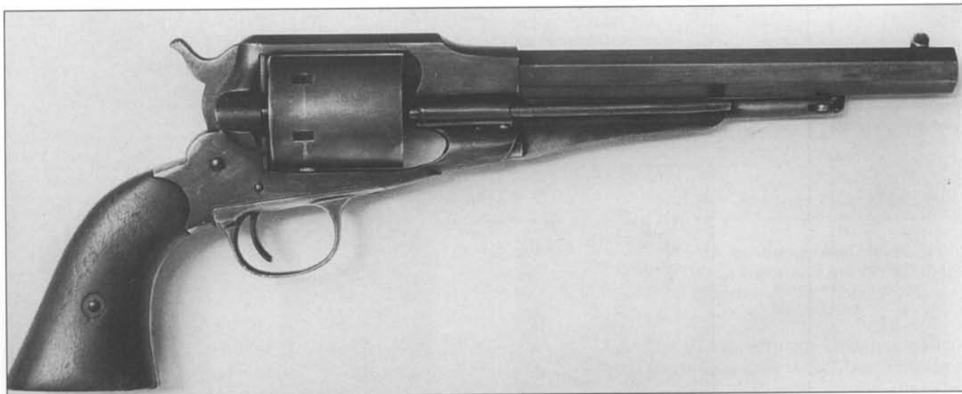
Fig. 3-59 Remington New Model Army revolver converted to six-shot, .44 caliber centerfire. serial number 119547. (Author's Collection)
