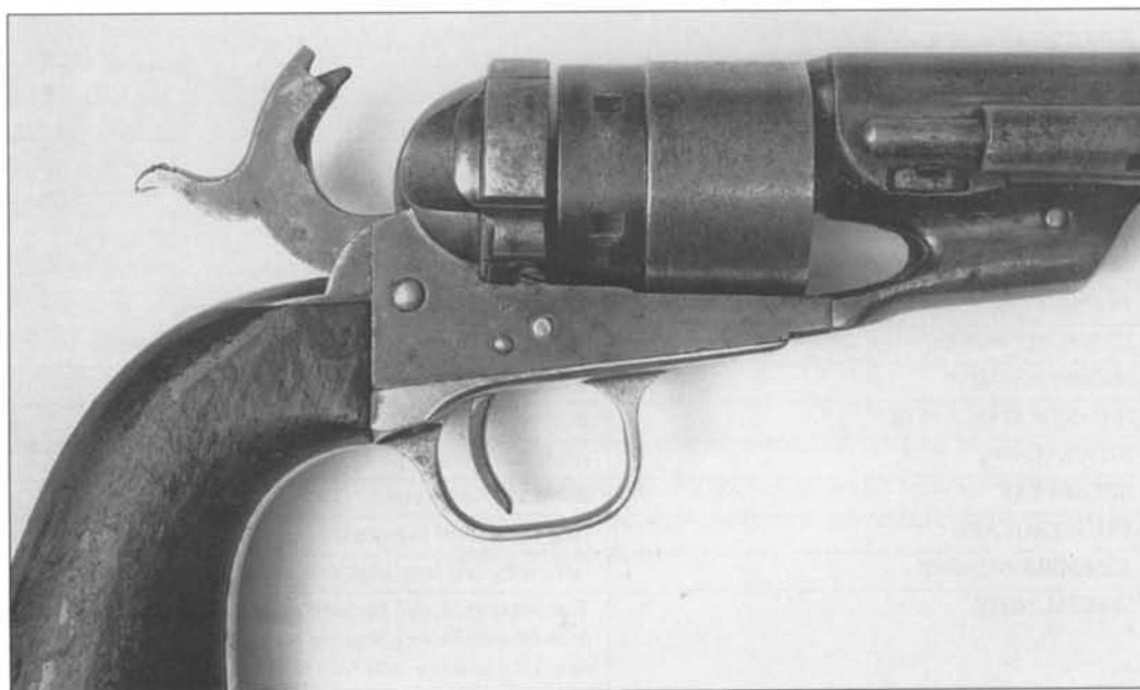
Fig. 5-75 Second Model Richards, serial number 194660, close-up of hammer, frame, cylinder, conversion ring and ejector rod tip. (Author's Collection)
