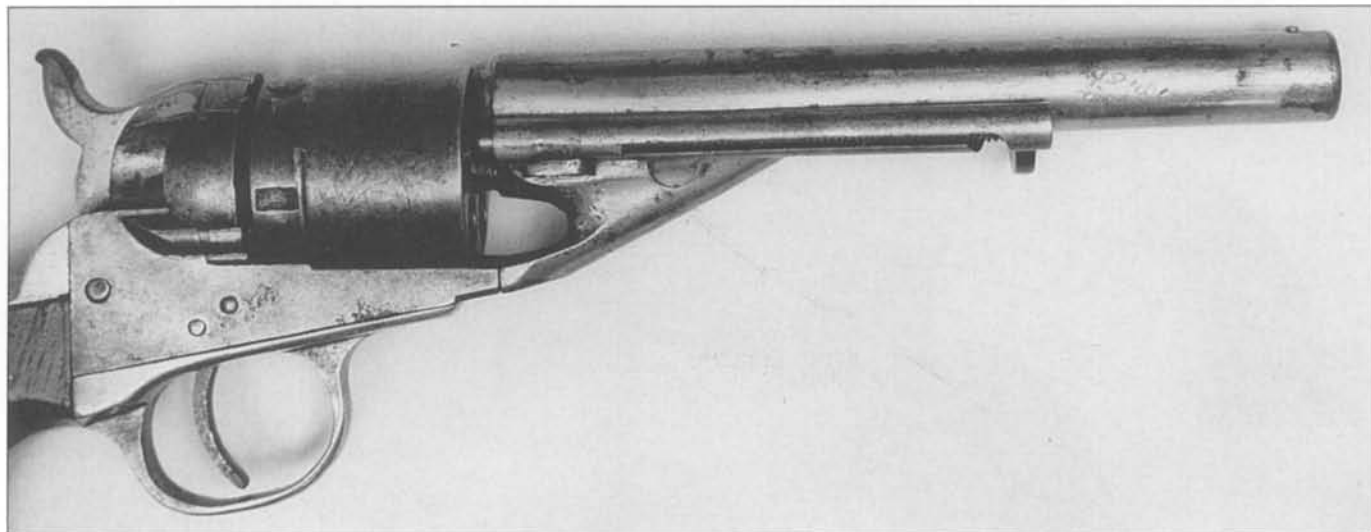
Fig. 8-26 Typical Colt Model 1862 Police conversion with round rebated cylinder and internal gate spring. Loading gates and cartridge ejector systems are common to all Model 1862 Police conversions, as illustrated.
