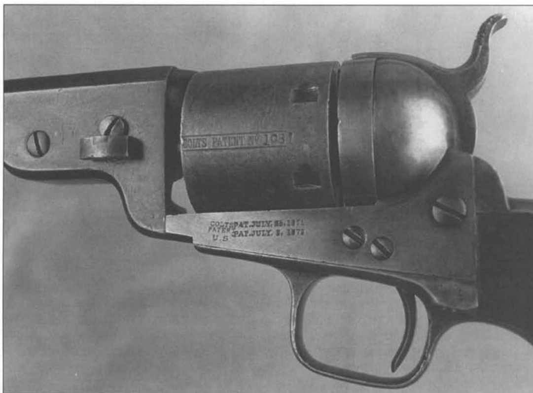
Fig. 6-69 Close-up of frame, barrel lug, cylinder and conversion ring of Colt Model 1851 Navy-Navy conversion showing two-line patent dates stamped to right of percussion frame stamp, with "U.S." remaining. Serial number 61769. (Courtesy Francis E. "Bud" Firth)
