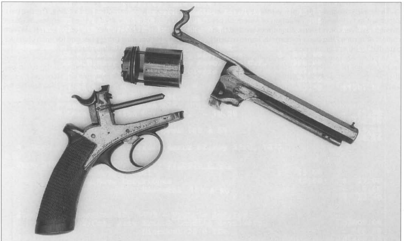
Fig. 10-12 Deane-Harding conversion revolver, broken open with cylinder removed.
