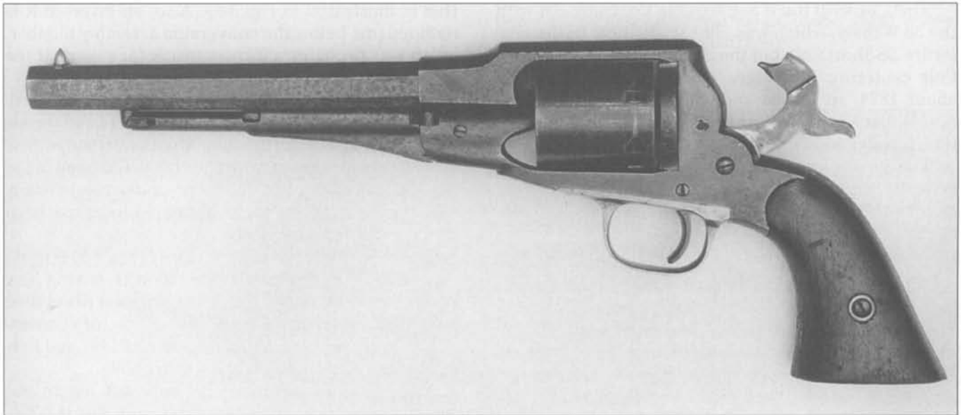
Top: Fig. 3-87 Remington New Model Navy revolver, factory converted to .38 caliber centerfire. Serial number 22378, conversion number 914. (Author's Collection)
