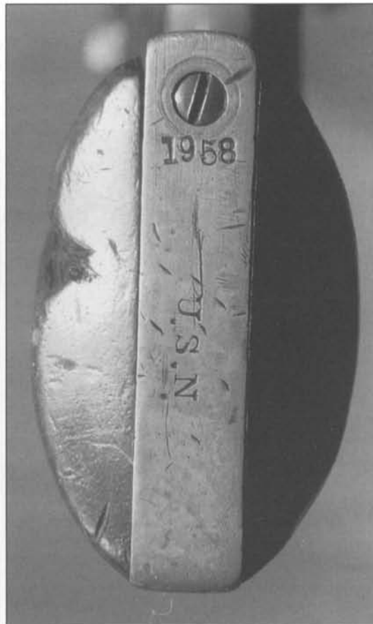
Above: Fig. 6-109 Close-up top view of barrel breech and cylinder of U.S. Navy Model 1861 Richards-Mason conversion, serial number 4158. The small anchor indicates reinspection while percussion. (Courtesy Francis E. "Bud" Firth)
