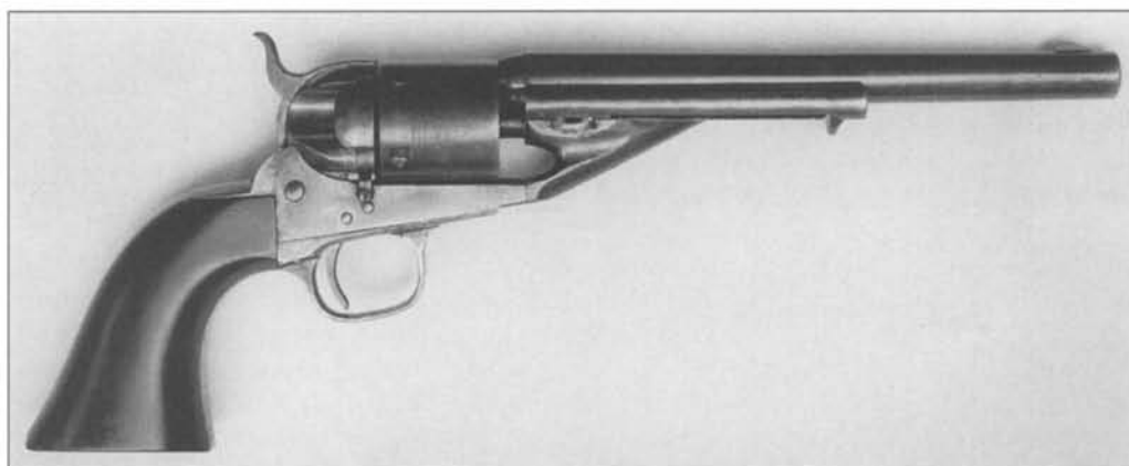
Fig. 6-86 Late production Colt Model 1861 Original Metallic Cartridge Richards-Mason revolver, serial number 2888. External gate spring. (Author's Collection)
