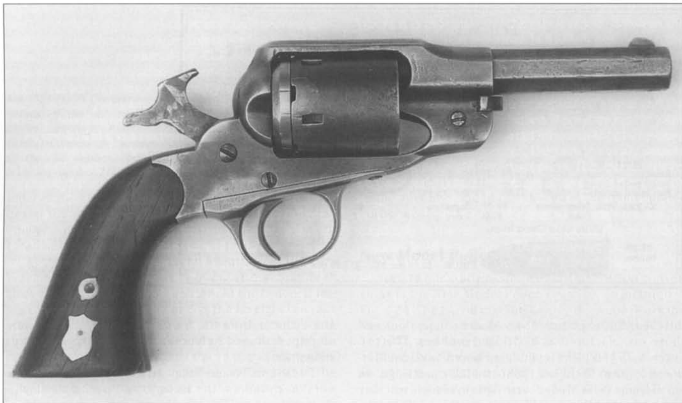
Fig. 3-26 Remington New Model Police revolver (non-factory) conversion to .38 centerfire. Serial number 15669. (Author's Collection)
