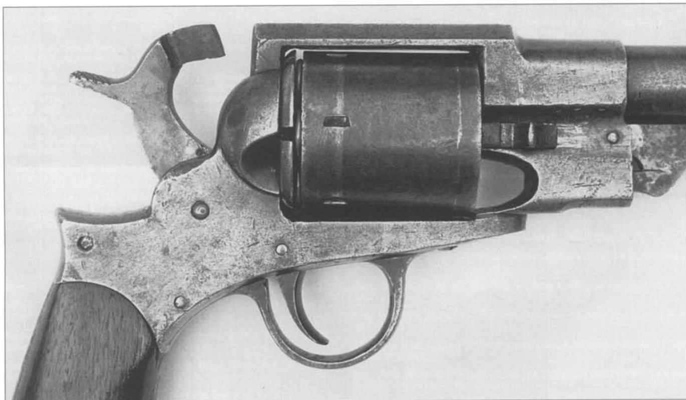
Fig. 10-21 Right side view of frame, cylinder, hammer, backing plate and thumbcatch of the Austin T. Freeman conversion.
