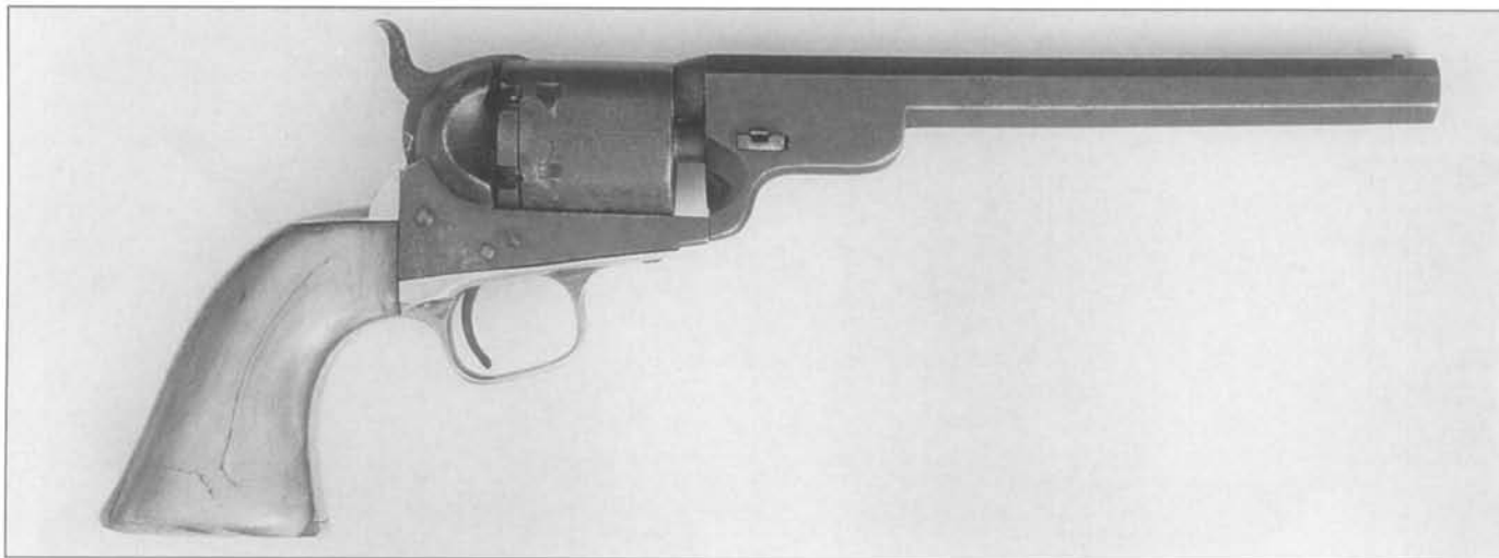
Fig. 9-21 Converted Model 1851 Colt Navy revolver with 2-piece cylinder. Serial number 112901. (Courtesy George R. Innocent)
