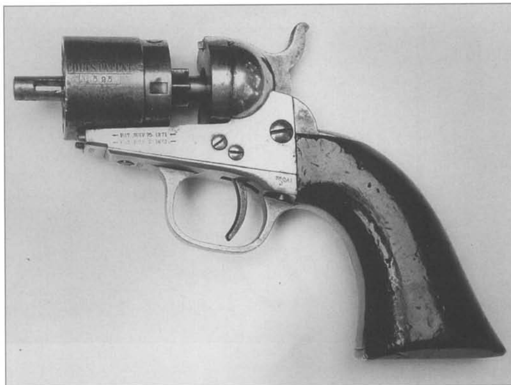
Fig. 8-82 3-1/2-inch Cartridge Barrel revolver with barrel removed and cylinder forward on arbor, showing ratchet shaft detail. Serial number 4525 (Author's Collection)
