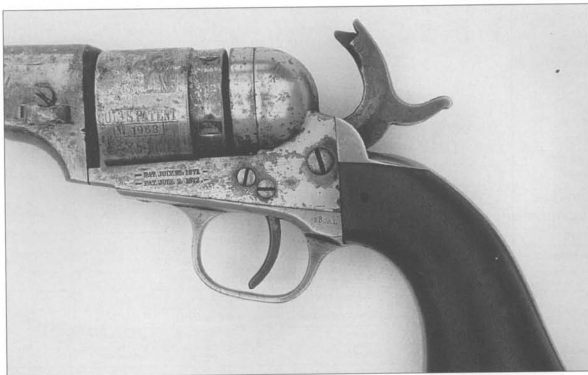
Fig. 8-90 Close-up of frame, cylinder and centerfire hammer of 3-1/2-inch Round Cartridge Barrel revolver, serial number 311963. (Author's Collection)
