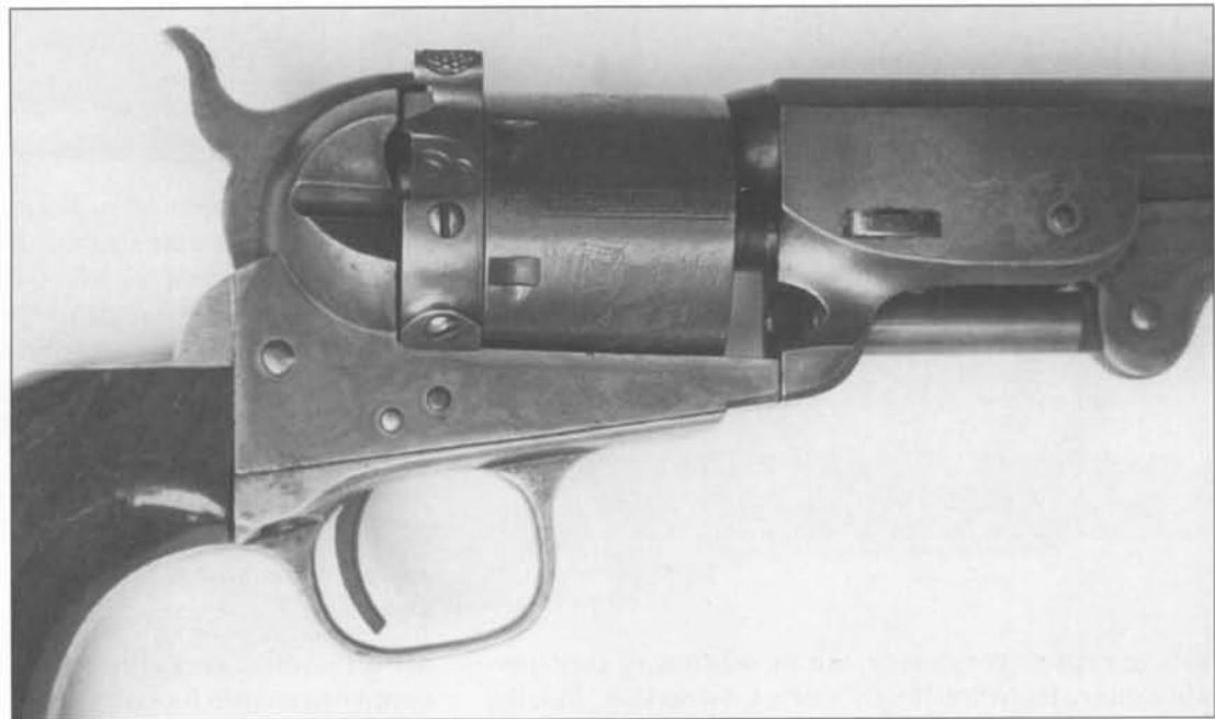
Fig. 4-5 Scooped out barrel lug loading channel of Hartford Colt Model 1851 Navy Thuer conversion.
