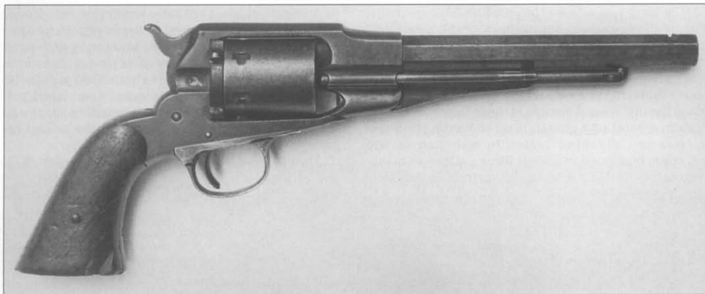
Fig. 3-91 Remington New Model Navy revolver, factory converted to .38 caliber centerfire. Serial number 25467, conversion number 630. (Author's Collection)
