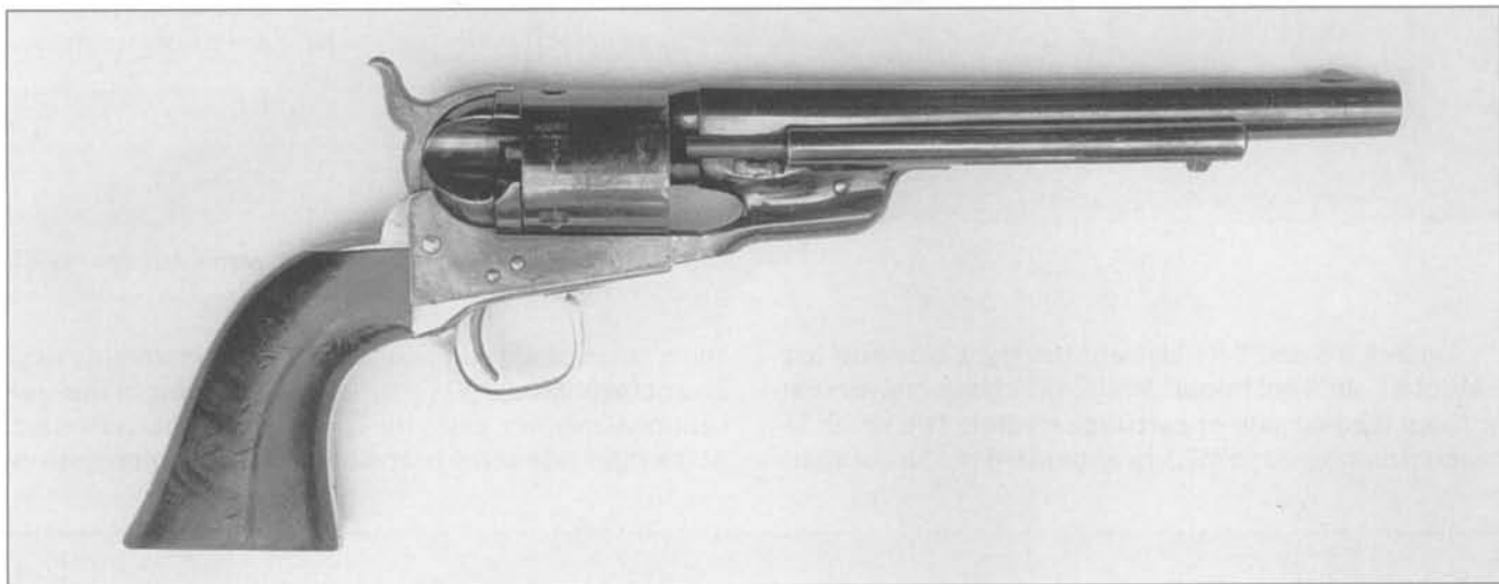
Fig. 9-12 Right side of experimental Model 1861 Navy conversion with 1860 Richards-style barrel and extractor. (Courtesy Francis E. "Bud" Firth)
