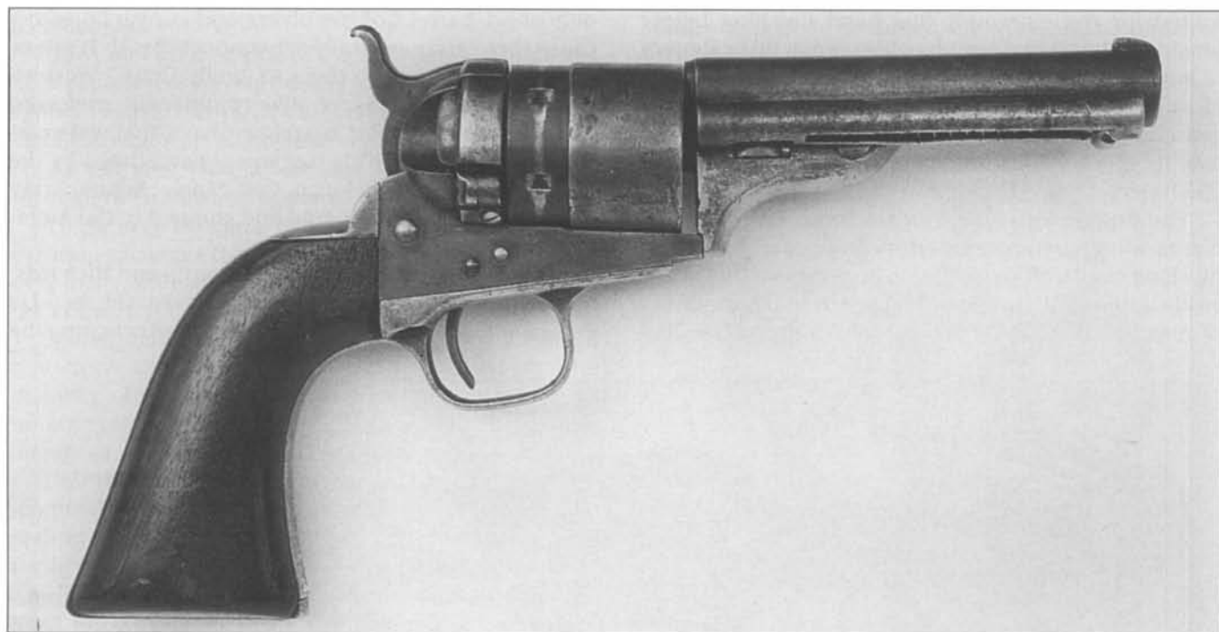
Fig. 9-38 Colt Model 1860 Richards-Mason conversion, serial number 6875, with barrel privately cut to 4-3/4 inches. (Author's Collection)
