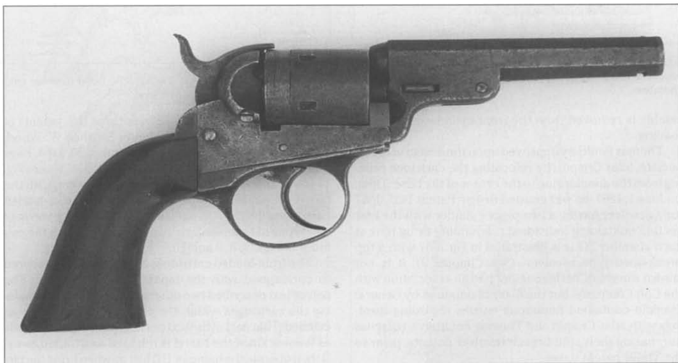
Fig. 4-35 Cooper Double Action Pocket conversion, serial number 501, with firing pin for each chamber of three-piece cylinder. (Author's Collection)
