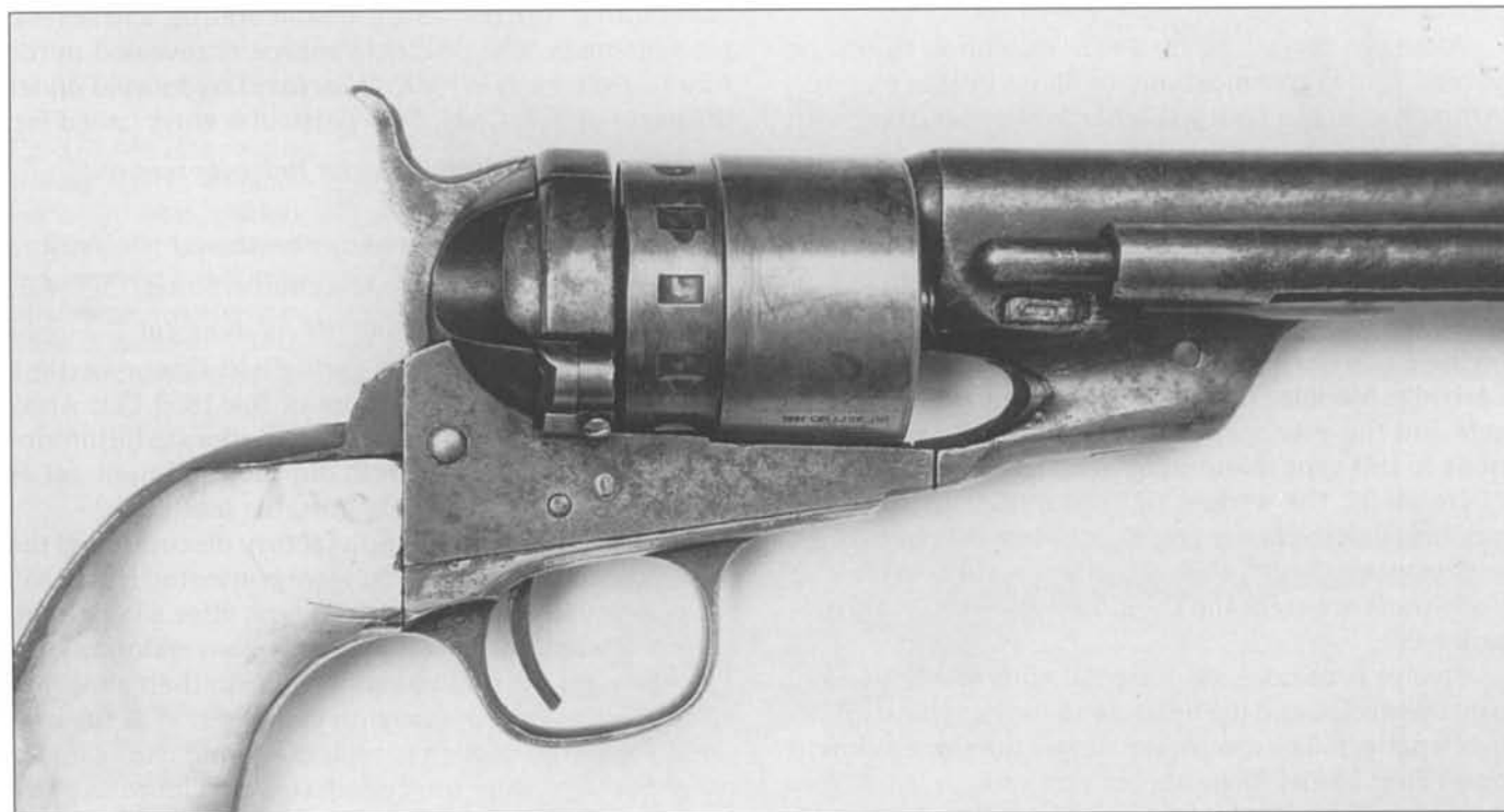
Fig. 5-71 Second Model Richards, serial number 198605, frame close-up, with 12-stop converted percussion military cylinder. (Author's Collection)
