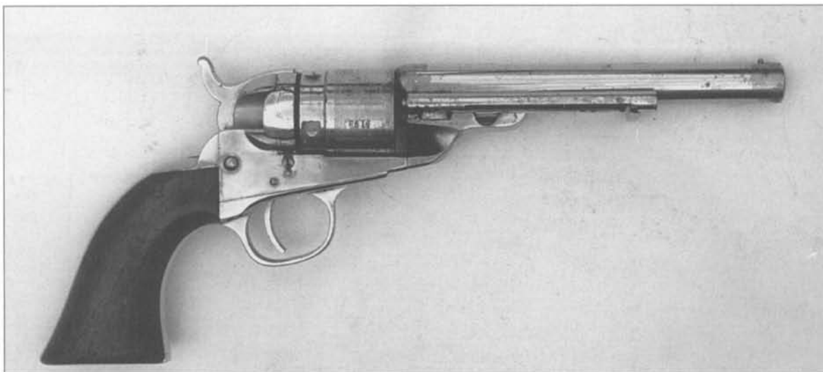
Fig. 8-73 Nickel Plated 5-1/2-inch Turned Round Barrel Colt Pocket Navy Cartridge revolver, serial number 3198, assembly number 3139. (Courtesy John H. Thillmann).
