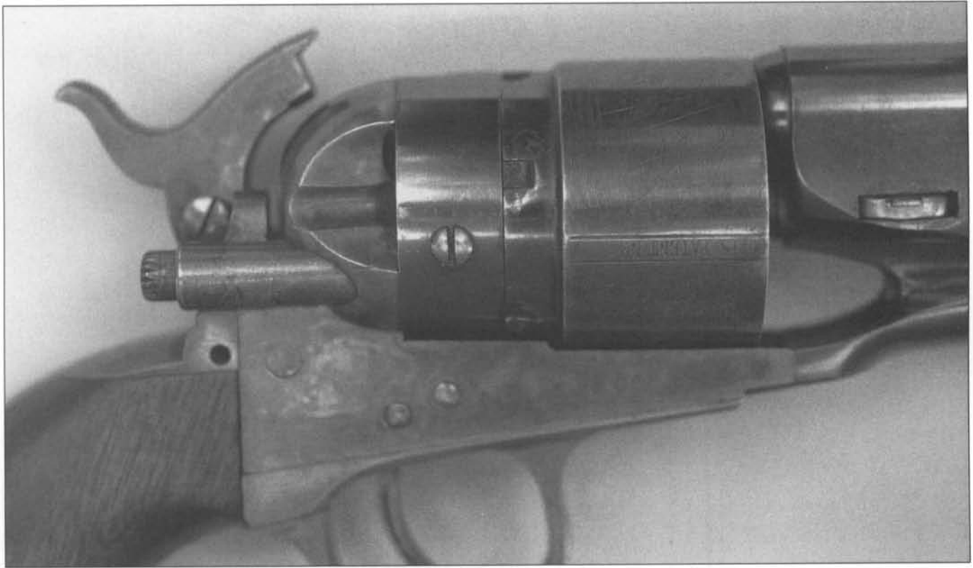
Fig. 4-41 Colt experimental 1860 Army revolver with hammer-operated cartridge ejector plunger. (Courtesy Museum of Connecticut History)
