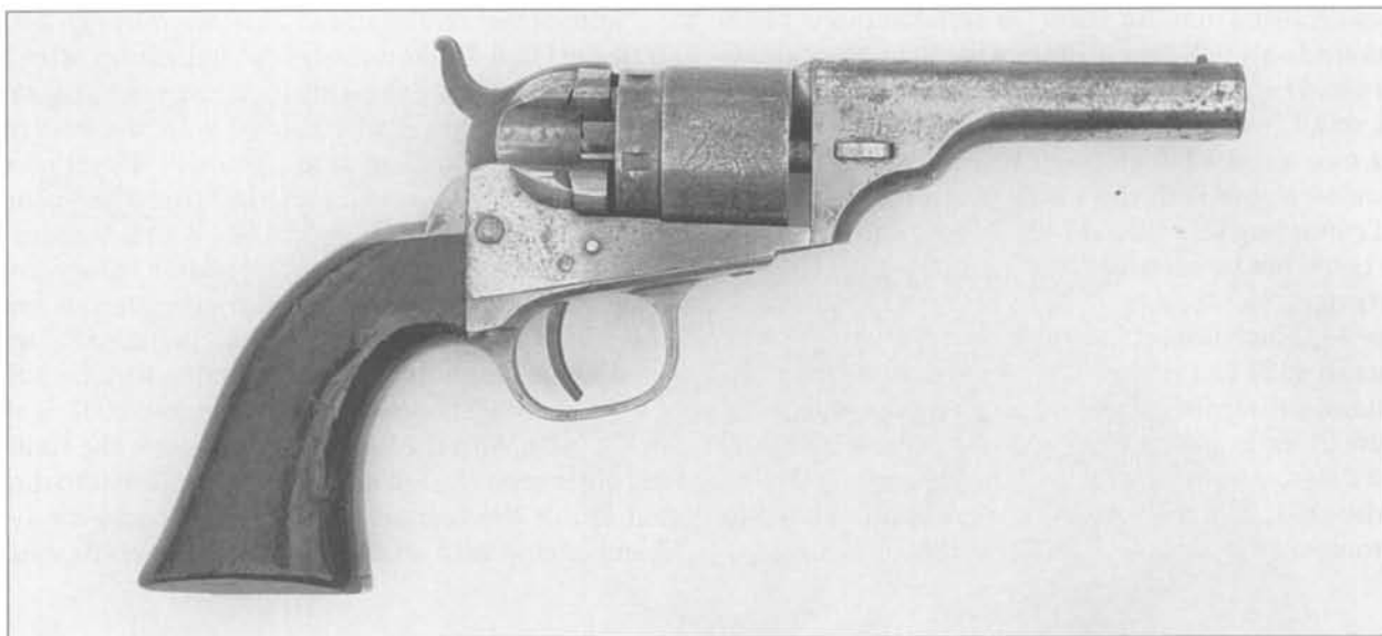
Fig. 8-85 Right side view of 3-1/2-inch Round Cartridge Barrel revolver, serial number 4525, showing detail of recut loading channel through recoil shield. (Author's Collection)
