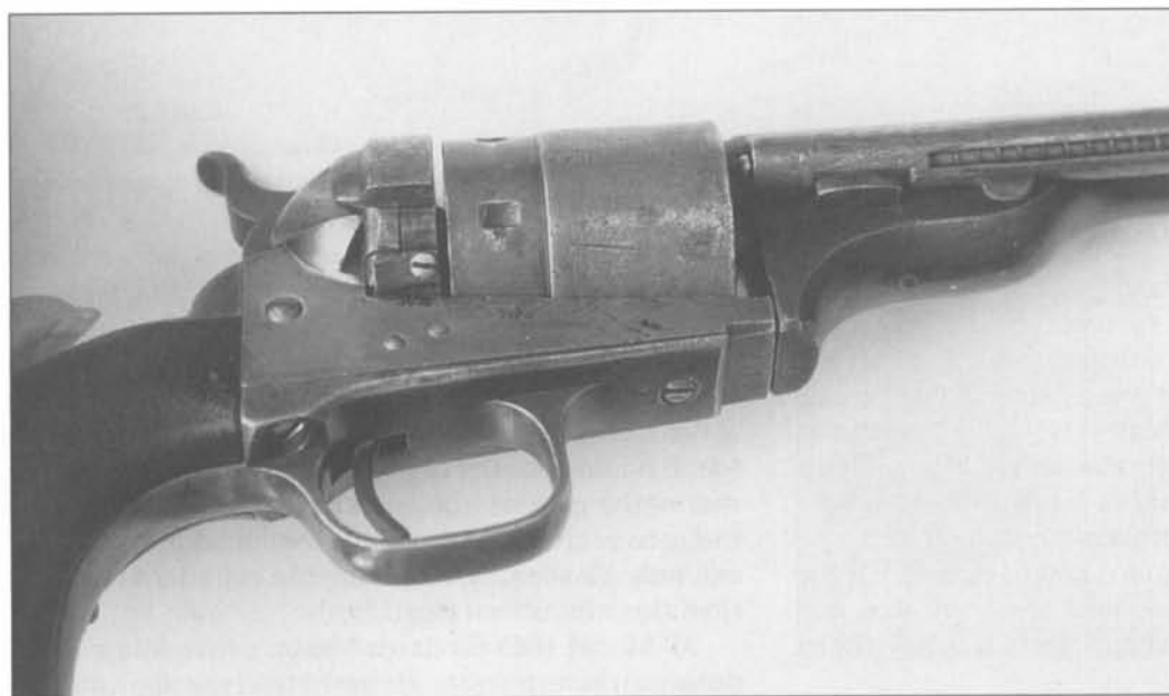
Fig. 6-10 Colt Model 1860 Richards-Mason conversion using percussion frame that has cut-outs at the recoil shield for shoulder stock. Serial number 7048, assembly number 1244. (Author's Collection)
