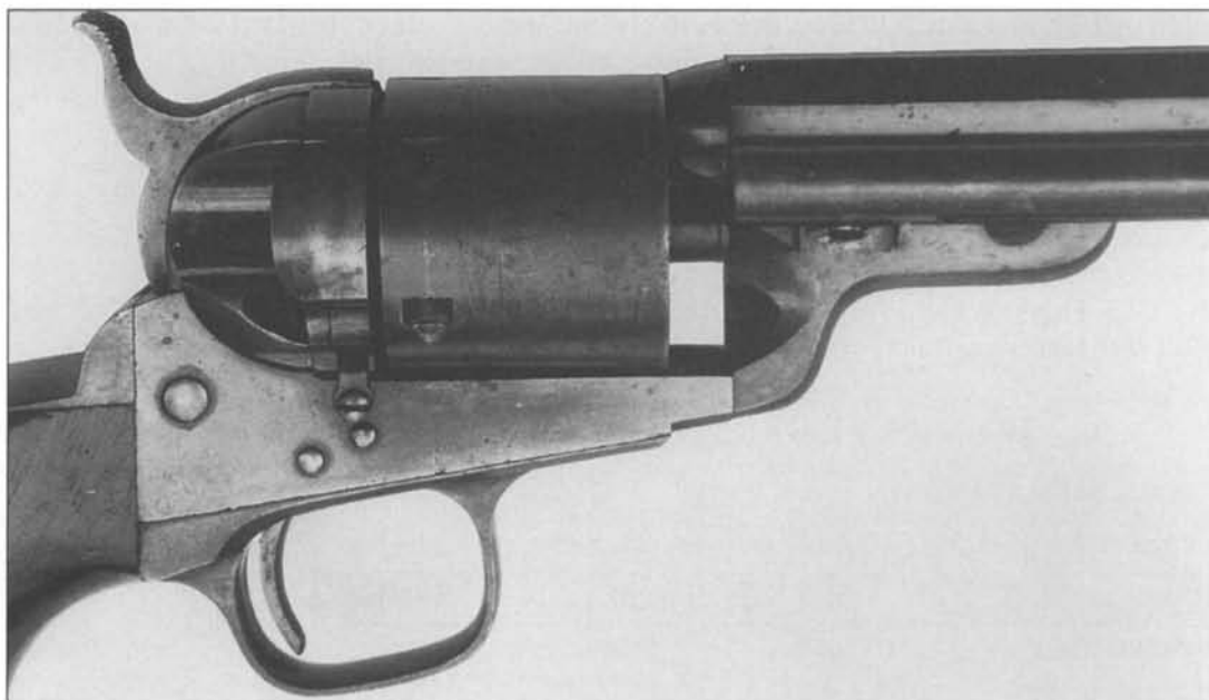
Fig. 6-60 Close-up of frame, barrel lug, cylinder and conversion ring of Model 1851 Navy-Navy conversion, serial number 89754. (Courtesy Dow and Russelle Heard)
