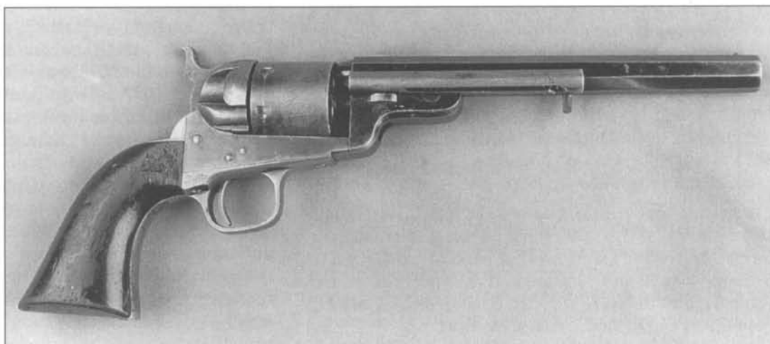
Fig. 6-50 Original Metallic Cartridge Colt Model 1851 Navy Richards-Mason revolver with newly fabricated barrel. Serial number 3170. (Courtesy Francis E. "Bud" Firth)
