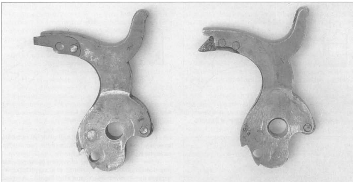
Fig. 8-16 Converted percussion hammers for rimfire (left) and centerfire (right) Colt small frame cartridge conversions.
