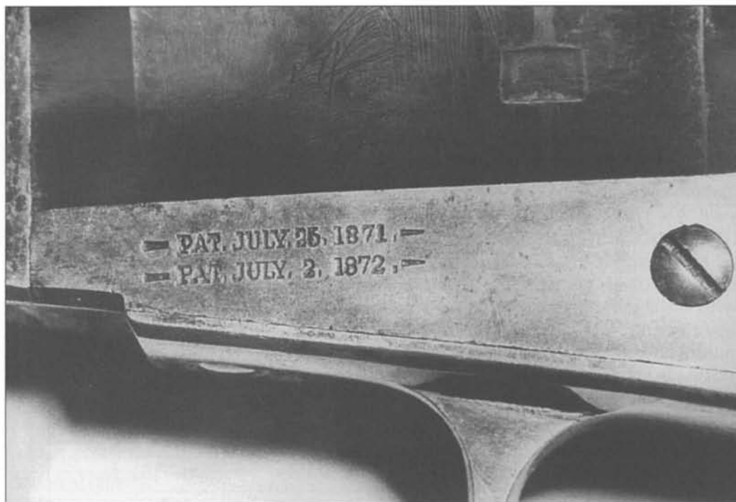
Fig. 6-40 Two-line patent dates typically stamped on new Colt Navy conversion frames, with dashes at the beginning and end of each line. (Author's Collection)
