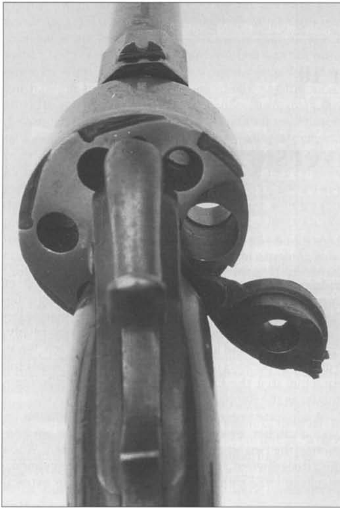
Fig. 10-2 Rear of Raphael breech-plate, showing cylinder chamber.
