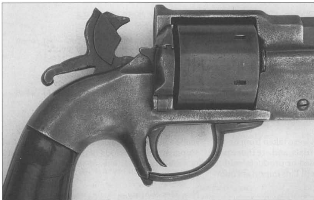
Fig. 10-54 Frame, cylinder, hammer and firing pin details of Allen & Wheelock Army conversion, serial number 181.
