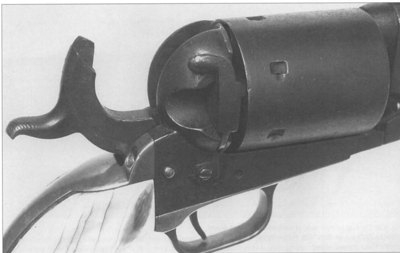
Fig. 9-32 Close-up showing frame, loading channel, gate, hammer-stop and cylinder of converted Dagoon, serial number 11907. (Author's Collection)
