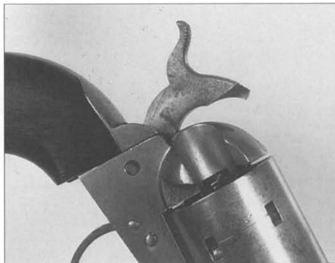
Fig. 9-60 Close-up of hammer, firing pin, and recoil shield with detail of loading channel of serial number 118000. (C.D. Terry Collection, photo by C.D. Terry and Francis E. "Bud" Firth)
