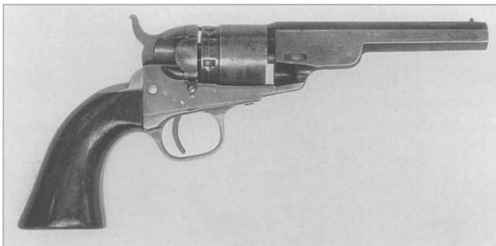
Fig. 8-56 4-1/2-inch Colt Pocket Navy Cartridge revolver with early production serial number (405), but external gate spring. (Courtesy John H. Thillmann)
