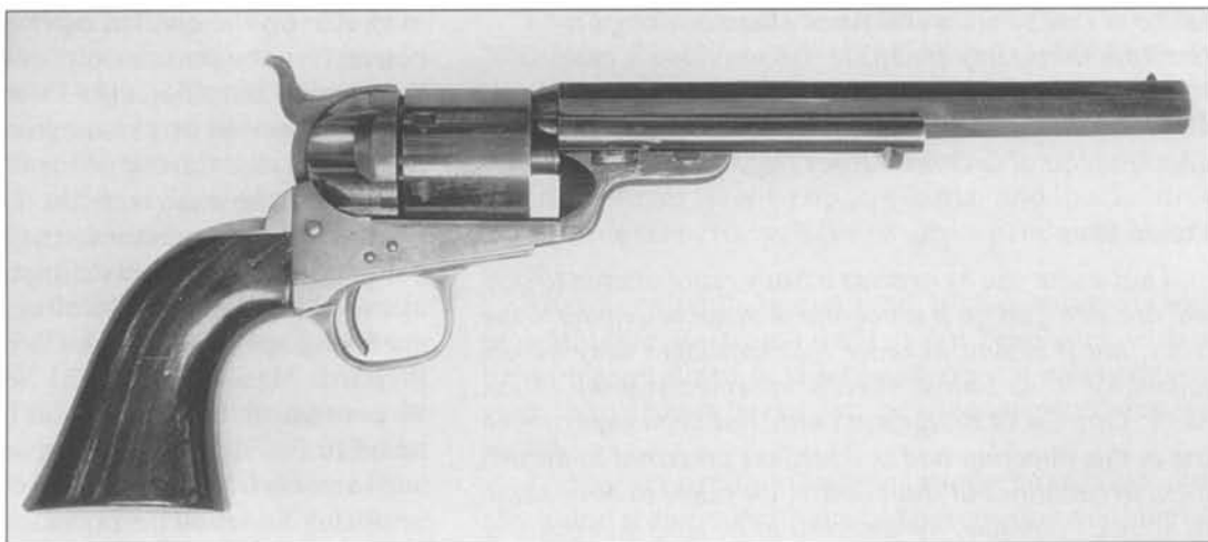
Fig. 6-49 Original Metallic Cartridge Colt Model 1851 Richards-Mason revolver with partially completed percussion barrel that has the lug bevel scooped out, but no "V" loading cut-out. Serial number 597, assembly number 1317. (Courtesy John H. Thillmann)
