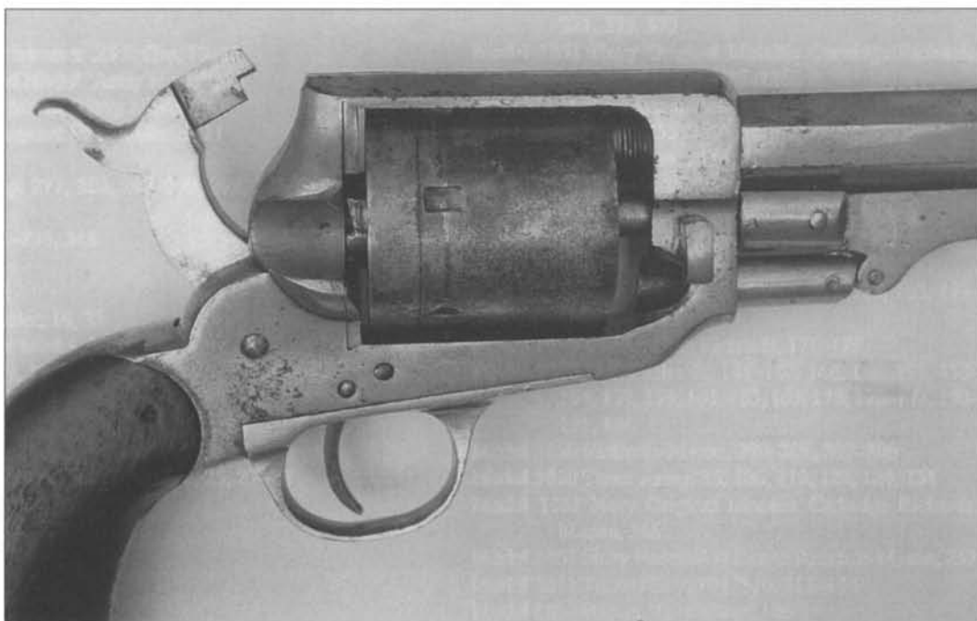
Fig. 10-28 Frame, cylinder, backing plate and hammer of the Whitney Navy revolver conversion.
