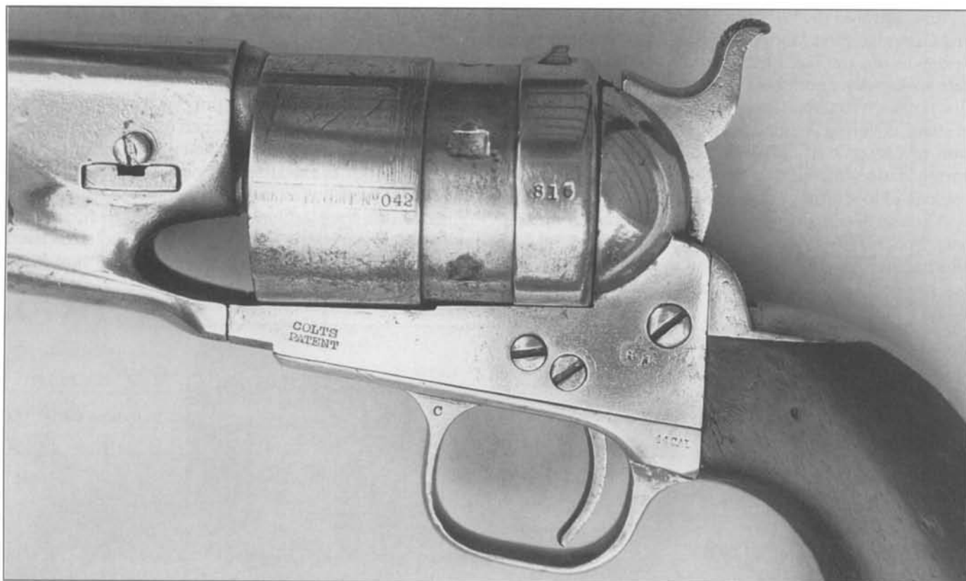
Fig. 5-38 First Model Richards close-up of frame, hammer, conversion ring and cylinder for assembly number 816, serial number 2042. (Author's Collection)
