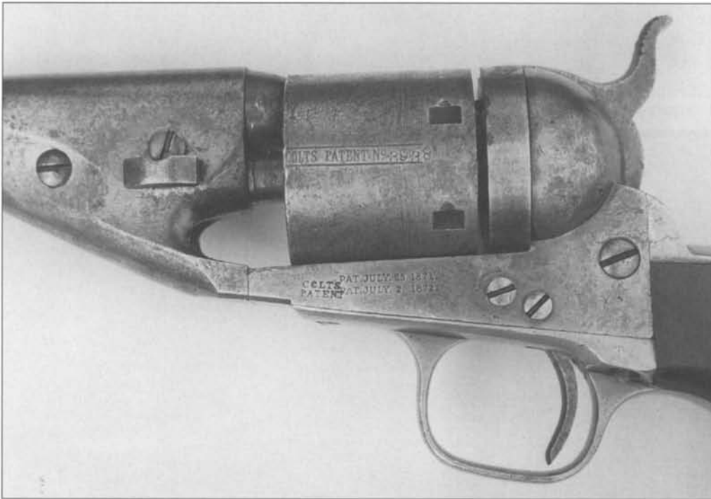
Fig. 6-98 Close-up of left side of Colt Model 1861 Navy conversion, serial number 6953, showing frame stampings and mismatched cylinder.
