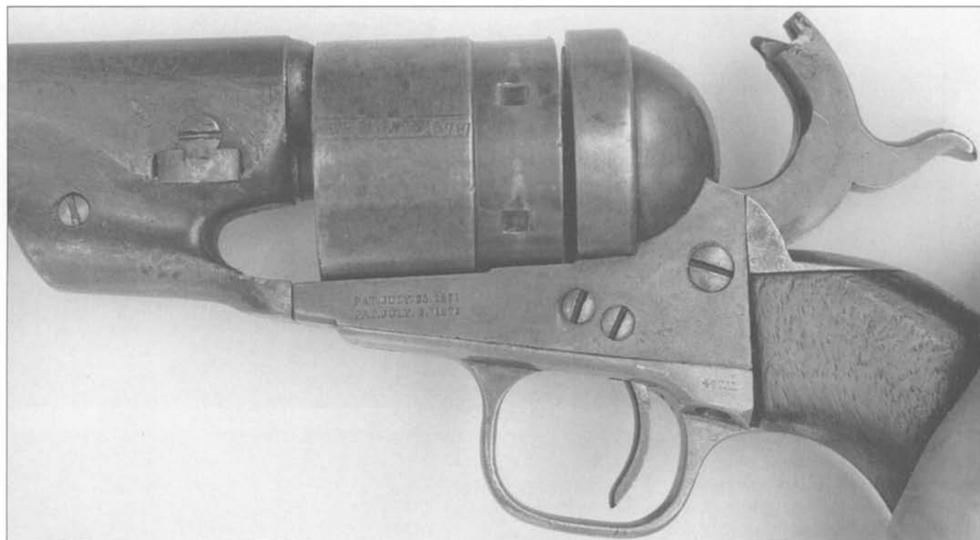
Fig. 5-84 Second Model Richards, serial number 196787; left side close-up of frame, hammer, cylinder and conversion ring.
