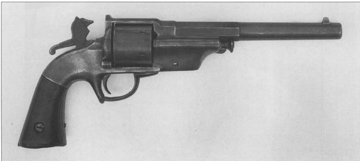
Fig. 10-53 Allen & Wheelock center-hammer Army revolver, serial number 181, converted to .44 Smith & Wesson Russian centerfire cartridge by refacing cylinder (see text). (Courtesy Martin D. Jessen)
