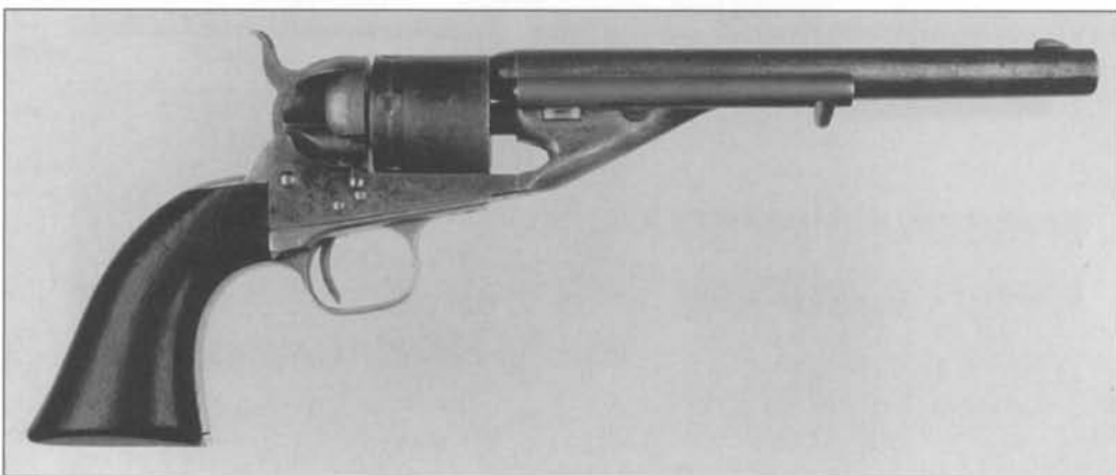
Fig. 6-108 U.S. Navy Colt Model 1861 Richards-Mason conversion, with original percussion Navy markings and reinspection markings. Serial number 4158, assembly number 918. (Courtesy Francis E. "Bud" Firth)
