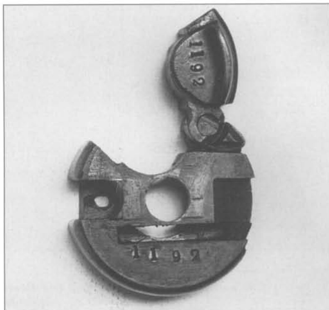
Fig. 6-14 Rear view of Colt Model 1860 Richards-Mason conversion ring with gate open, assembly number 1192. (Author's Collection)
