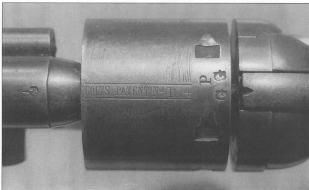
Fig. 6-112 Close-up top view of barrel breech and cylinder of U.S. Navy Model 1861 Richards-Mason conversion showing percussion reinspection stampings of serial number 7104. (Photo by L. Frank Richey, Sam Pachanian Collection)
