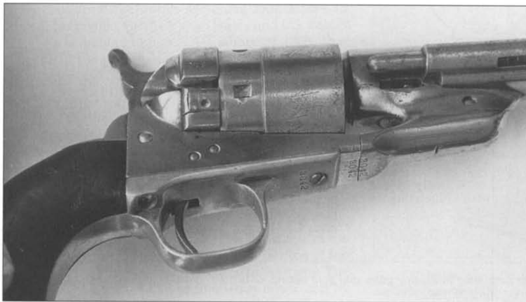
Fig. 5-33 First Model Richards, serial number 2042, assembly number 816. Frame close-up showing gate hinge with internal gate spring. (Author's Collection)
