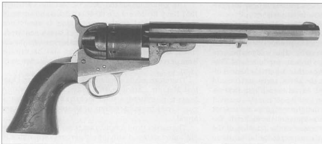
Fig. 6-46 Original Metallic Cartridge Colt Model 1851 Richards-Mason revolver with newly fabricated barrel with no lug cut-outs. Serial number 437, assembly number 684. (Courtesy Dow and Russelle Heard)
