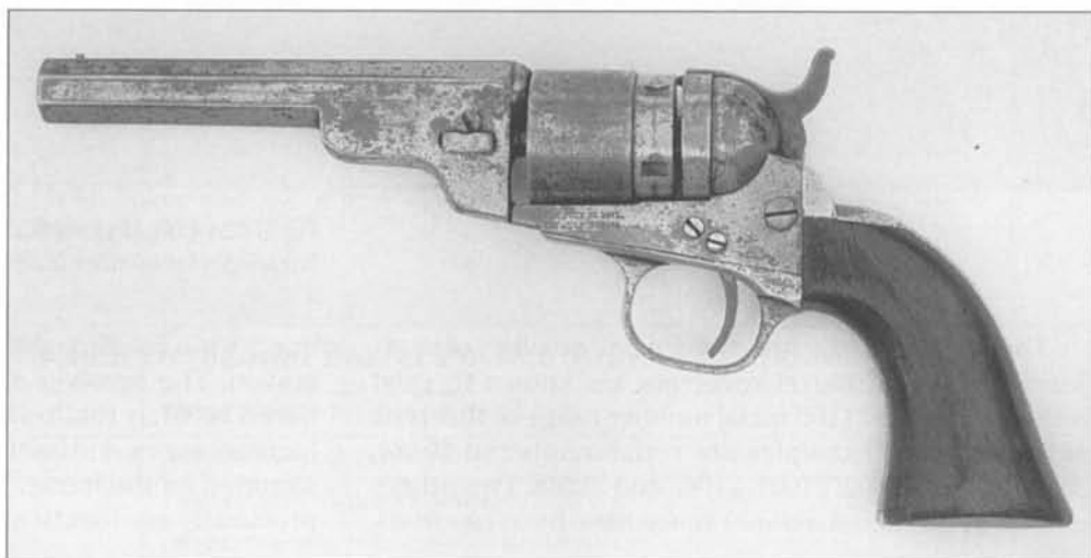
Fig. 8-65 4-1/2-inch Colt Pocket Navy cartridge revolver originally rimfire and converted to centerfire. Serial number 626, assembly number 510. (Author's Collection).
