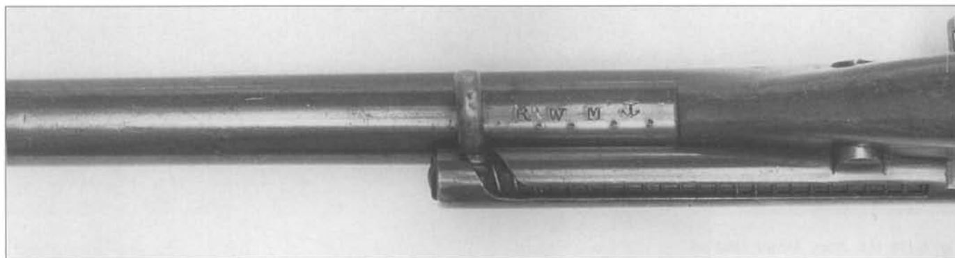
Above: Fig. 6-118 Underside of barrel of U.S. Navy Model 1861 Richards-Mason conversion with New York Navy Yard conversion inspector's stamp. Frame serial number 6957.
