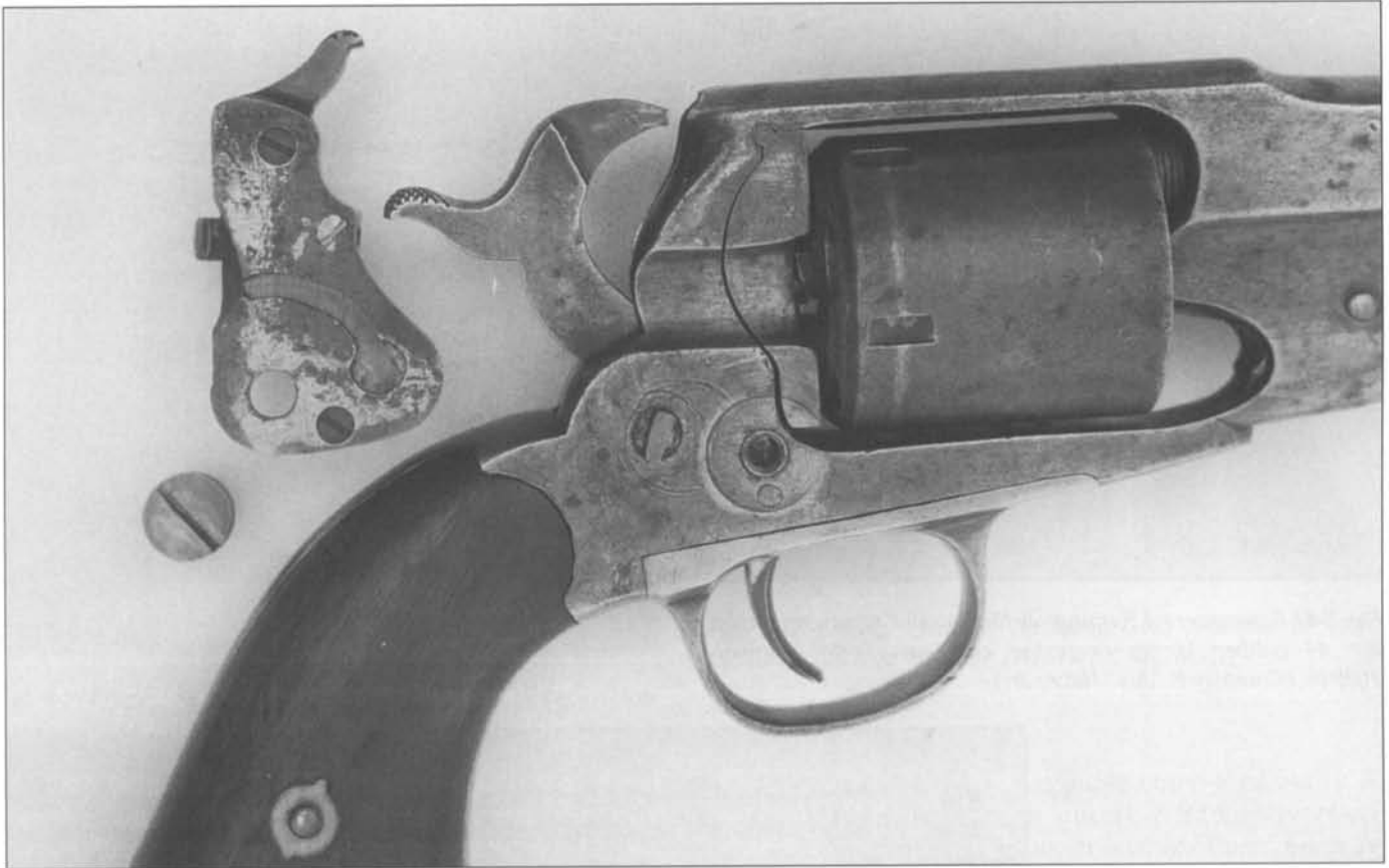
Fig. 3-42 Remington New Model Army Mason conversion, extractor detail.
