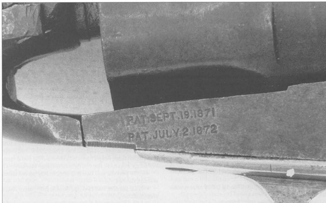
Fig. 8-100 Early Colt Single Action Army revolver frame stamping found on a limited number of late Colt small frame conversions.
