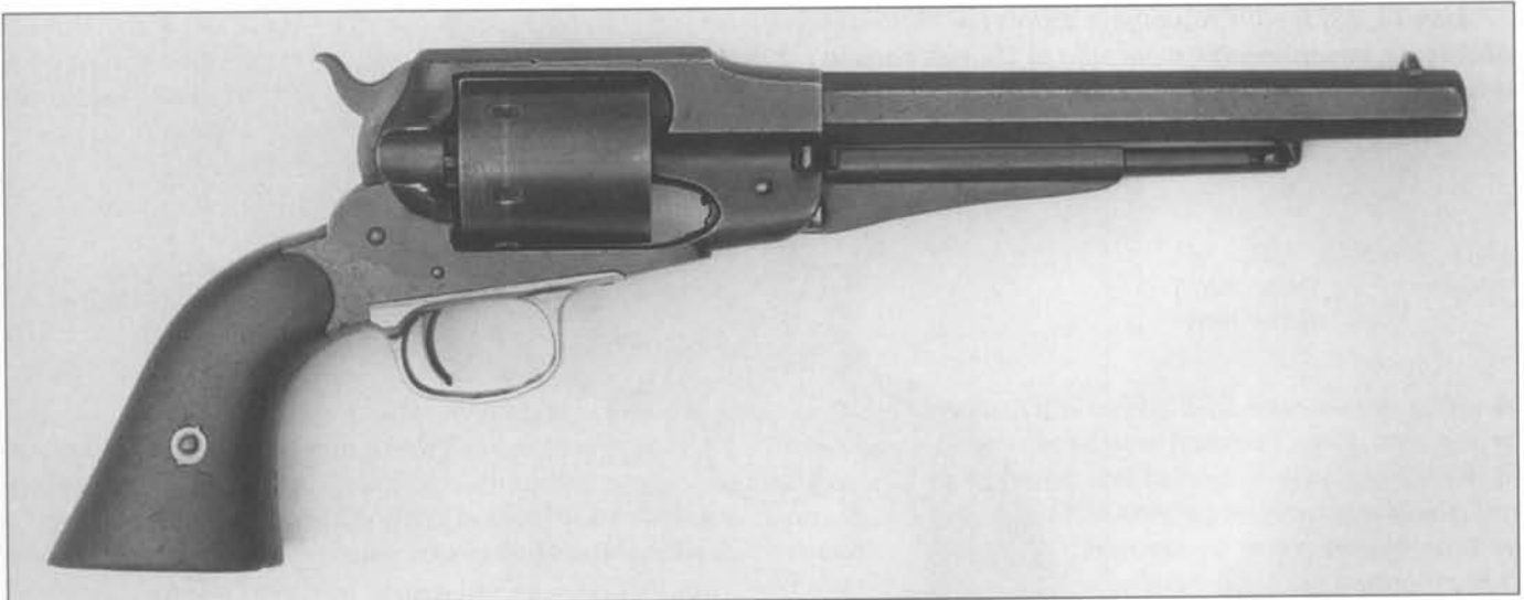
Fig. 3-66 Remington New Model Army revolver conversion with welded back-plate. Serial number 93609, conversion number 1151. (Author's Collection)
