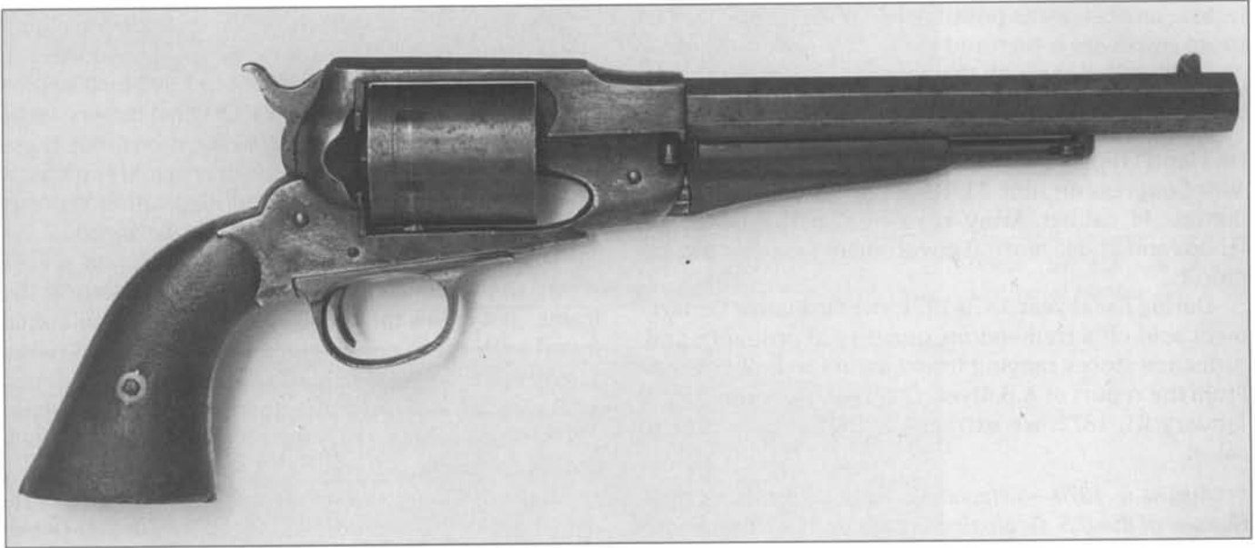
Fig. 3-65 Remington New Model Army revolver, armory conversion in .44 caliber cylinder made of two pieces. Serial number 90,261. (Author's Collection)
