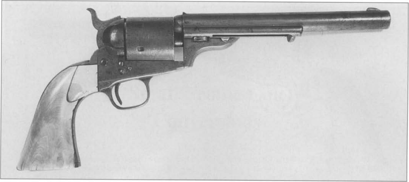
Fig. 7-36 Colt Model 1871-1872 Open Top revolver, serial number 3119, with ivory grip. (Author's Collection)
