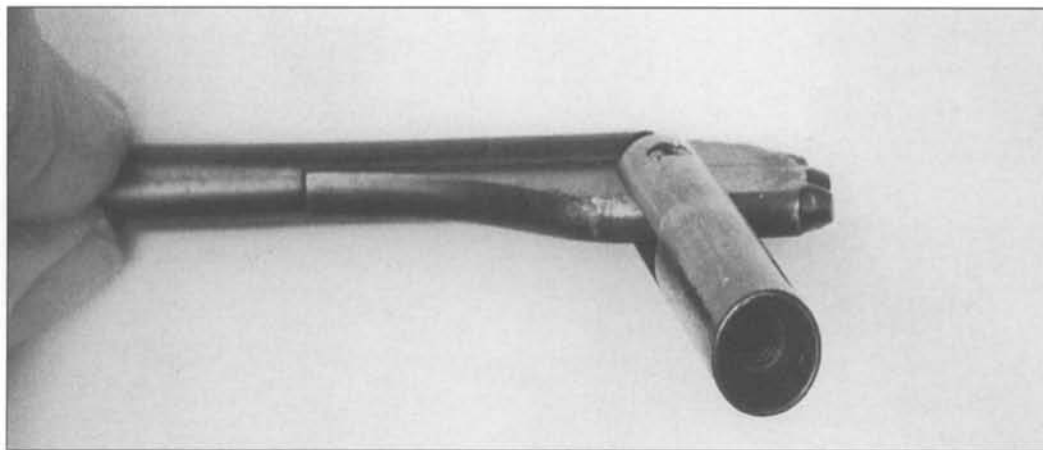
Fig. 4-2 1860 Colt Army Thuer plunger, drilled and threaded to accept the Thuer priming punch (see Figs. 4-23 through 4-25).
