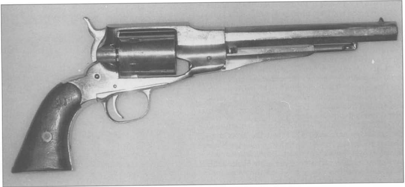
Fig. 3-76 Armory converted Remington Model 1861 Navy revolver. Serial number 16244. Cylinder is stamped PAT.APP'D FOR. (Author's Collection)
