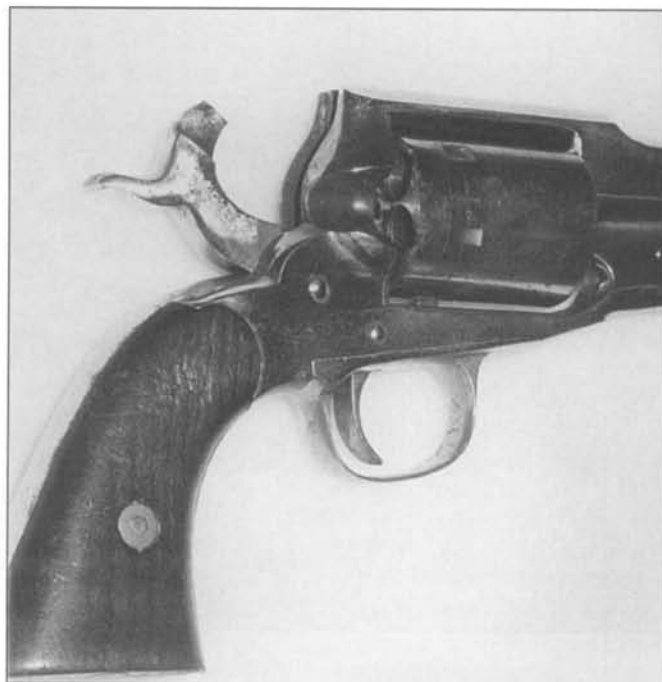
Fig. 3-78 Frame of Model 1861 Navy conversion, serial number 16244 showing the cartridge flange recesses.
