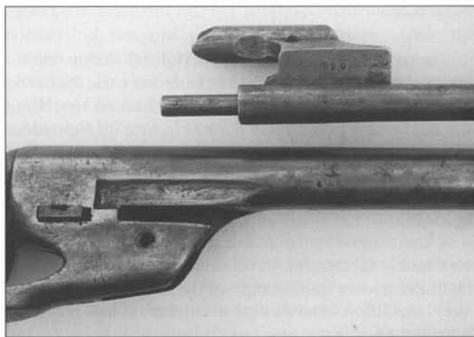
Fig. 5-3 U.S. Richards barrel and ejector housing, assembly number 622. (Author's Collection)
