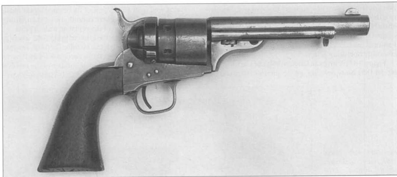
Fig. 9-40 Colt Model 1860 Richards-Mason conversion with barrel privately cut to 5-3/8 inches. Serial number 5975. (Author's Collection)
