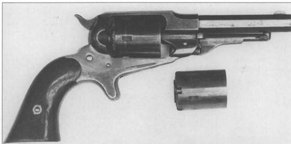
Fig. 3-17 Remington New Model Pocket revolver with the original percussion cylinder and conversion cylinder with back-plate. Serial number 21943, conversion assembly number 3683. (Author's Collection)
