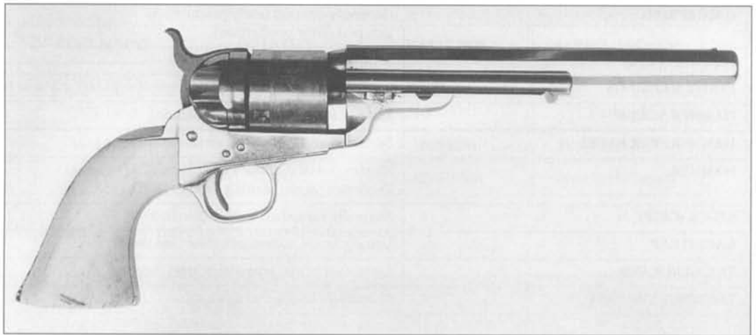
Fig. 6-44 Original Metallic Cartridge Colt Model 1851 Richards-Mason revolver, full nickel plated with ivory grips, and partially completed percussion barrel. Serial number 1790, assembly number 3340. (Courtesy Dow and Russelle Heard)
