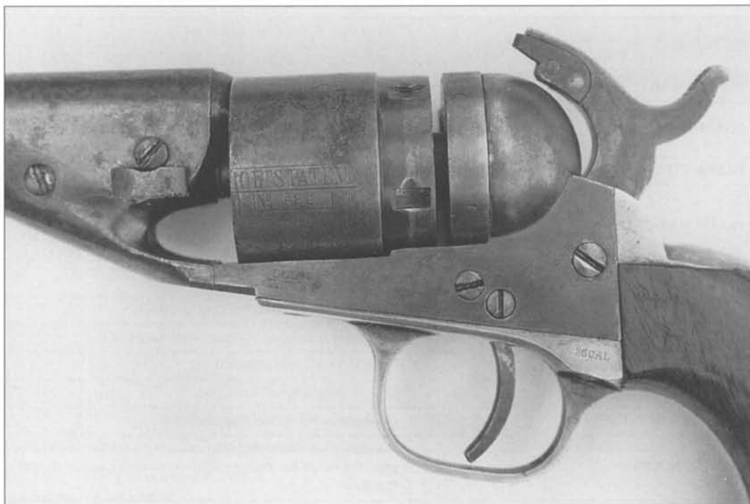
Fig. 8-27 Early production Colt Model 1862 Police Cartridge revolver with COLT'S/PATENT frame marking; rimfire ignition, serial number 2682. (Author's Collection)
