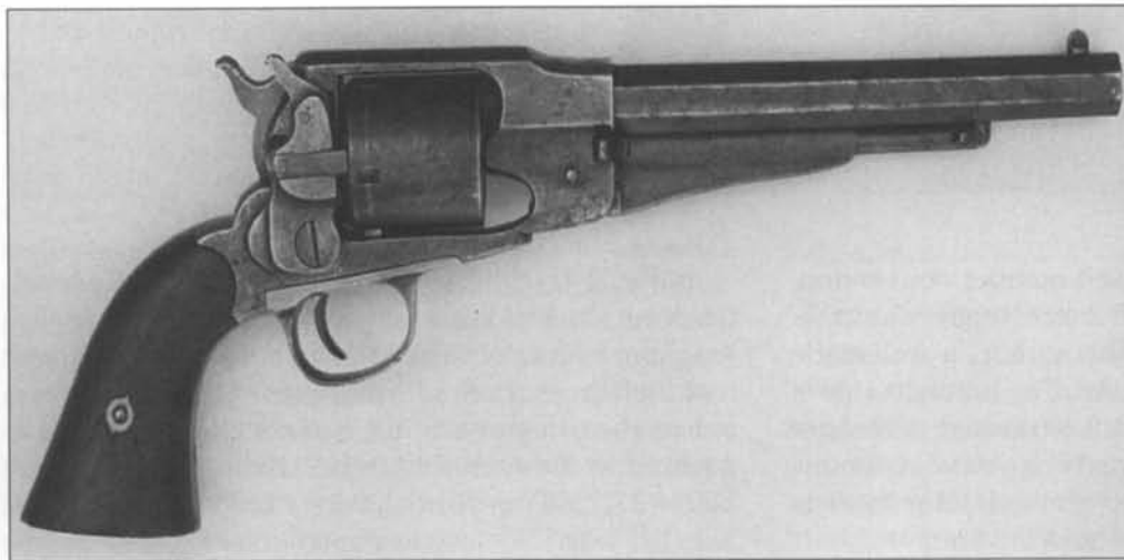
Fig. 3-39 Remington New Model Army Revolver conversion with W. Mason Cartridge extractor. Serial number 152999 (frame) and 129283 (barrel). (Author's Collection)
