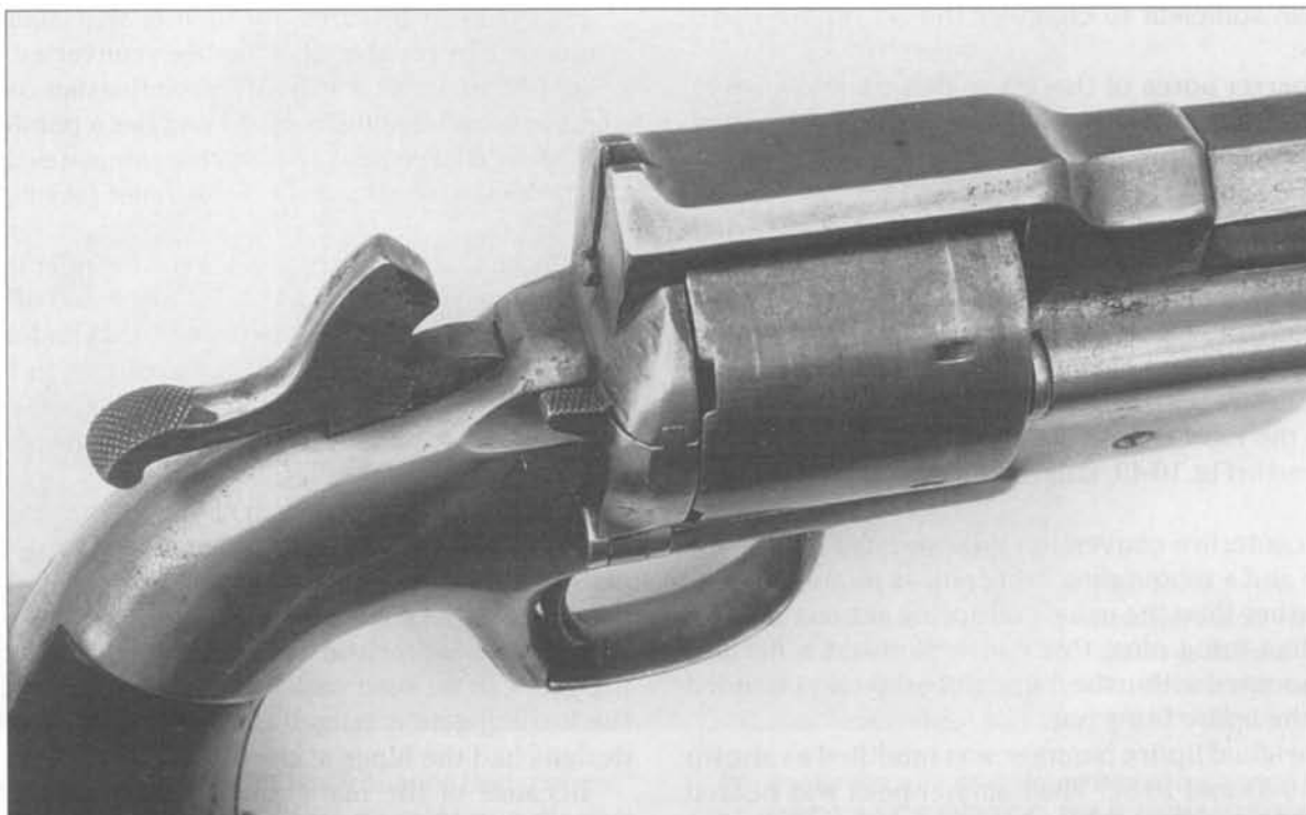
Fig. 10-51 Frame, cylinder and hammer detail of Allen & Wheelock Army centerfire conversion, serial number 96.
