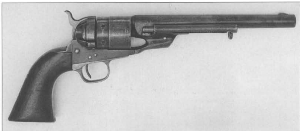
Fig. 5-81 Second Model Richards, serial number 196787, assembly number 6787, with "doughnut" ejector head. (Author's Collection)
