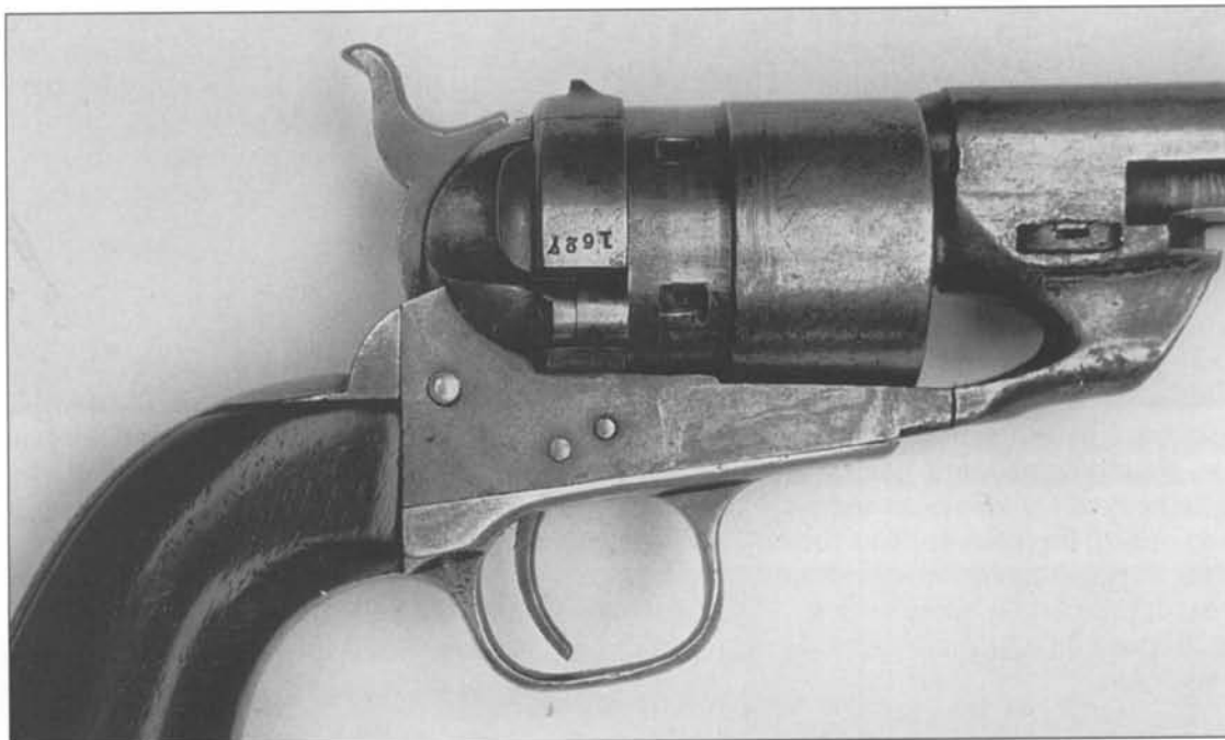
Fig. 5-36 First Model Richards close-up of conversion ring numbered on outside with the assembly number 1627. (Author's Collection)
