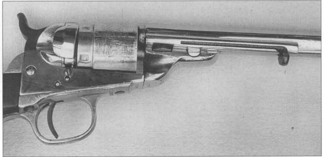
Fig. 8-4 Mason ejector assembly mounted on Turned Round Barrel Colt Pocket Navy conversion, serial number 12272.
