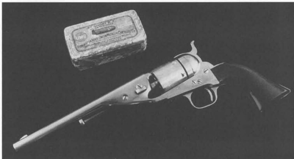
Fig. 6-84 Colt Model 1861 Original Metallic Cartridge Richards-Mason revolver pictured with a box of .38 Short rimfire cartridges by U.M.C. Serial number 1132/1 (Courtesy Francis E. "Bud" Firth)
