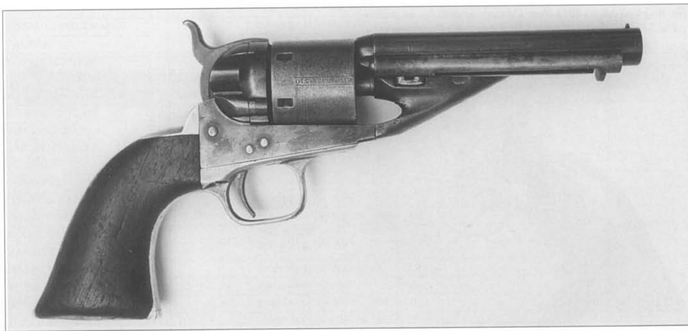
Fig. 9-44 Colt Model 1861 Navy Conversion with barrel privately cut to 4-13/16-inches. Serial number 1510. (Author's Collection)
