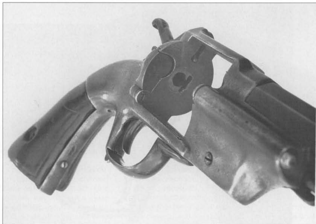
Fig. 10-49 Enlarged loading channel of Allen & Wheelock Army conversion caused misfit of gate to frame.
