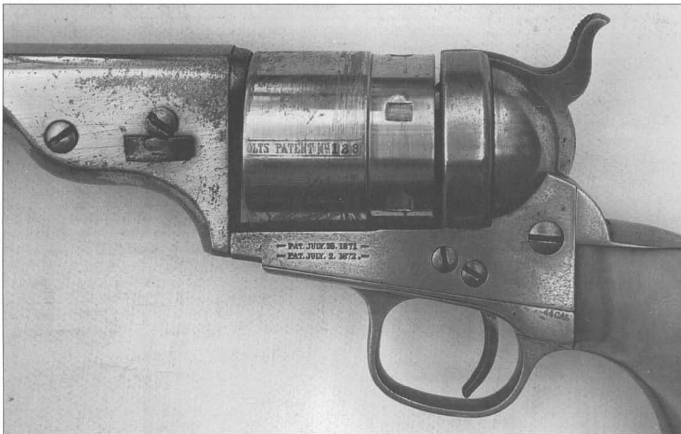
Fig. 6-8 Close-up of nickel-plated Model 1860 Richards Mason frame and cylinder, showing frame markings and cylinder number 123 matching that of the gun, 7123. (Courtesy John H. Thillmann)
