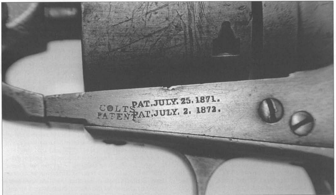
Fig. 6-39 Two-line patent dates stamped to the right of the original percussion frame stamping on a U.S. Model 1861 Navy-Navy conversion, serial number 4154 (mixed). (Courtesy Francis E. "Bud" Firth)
