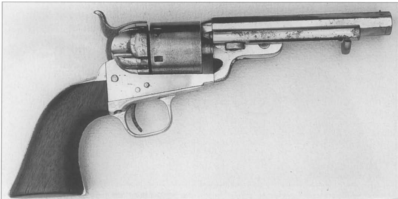
Fig. 9-41 Colt Model 1851 Navy conversion, serial number 103, with barrel privately cut to 4-5/8 inches. (Author's Collection)
