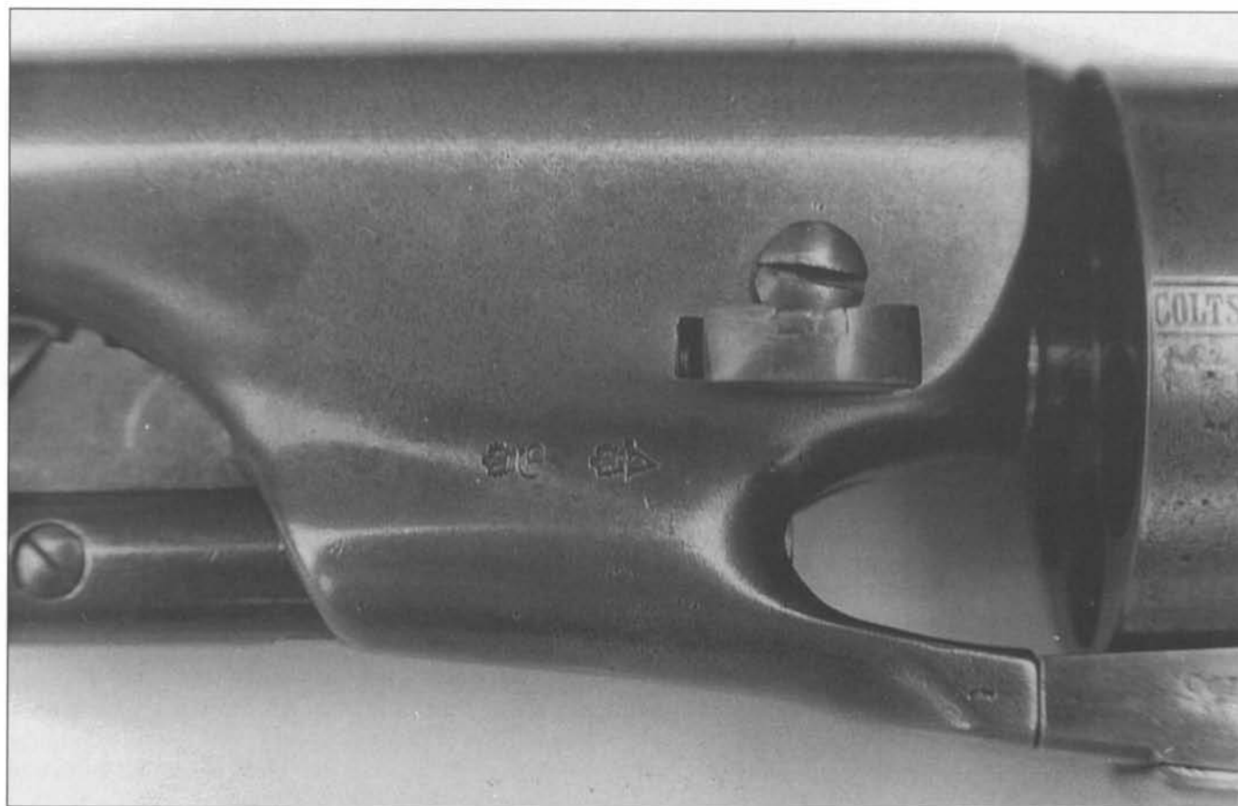
Fig. 4-75 British proof marks of the early 1860s found on the barrel lug of 1860 Army Thuer conversion, serial number 95123. (Courtesy Francis E. "Bud" Firth)
