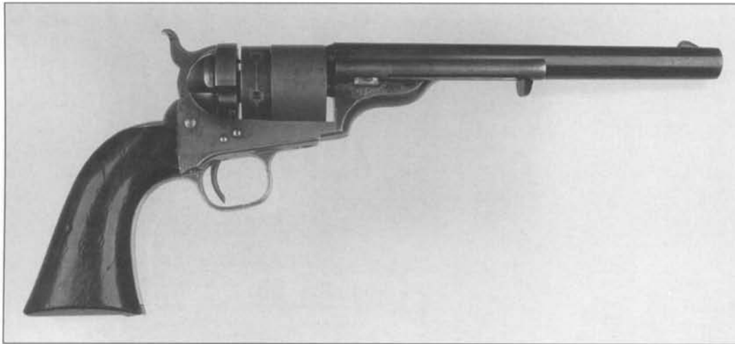
Fig. 6-17 Colt Model 1860 Richards-Mason newly fabricated wedge, without spring. (Author's Collection)
