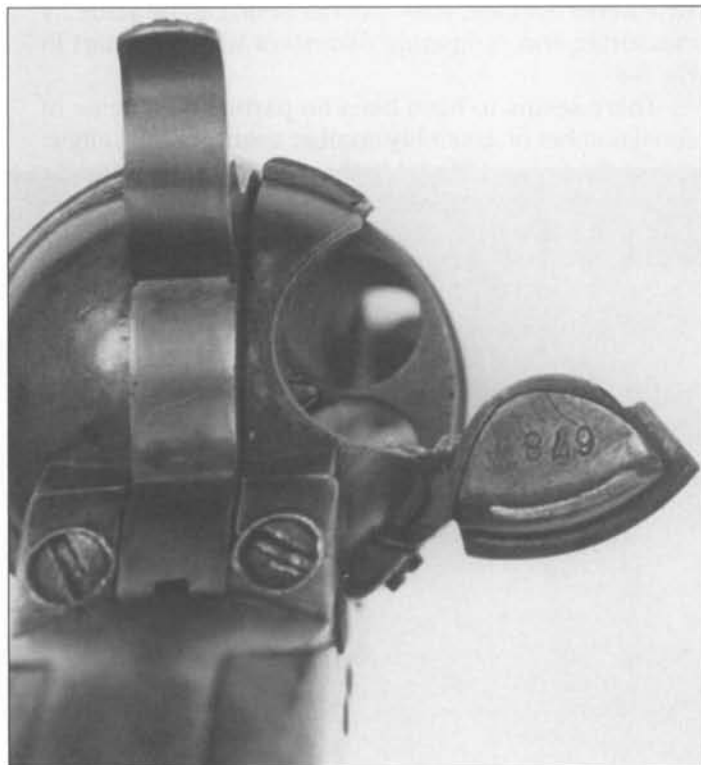
Fig. 5-83 Second Model Richards, serial number 196787; close-up showing assembly number in rear of the loading gate.
