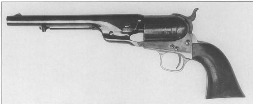
Fig. 6-93 Factory experimental Model 1861 Richards-Mason conversion. Left side view shows there are no frame markings. The gun is unnumbered and the barrel address is the New York Type II. (Courtesy Francis E. "Bud" Firth)
