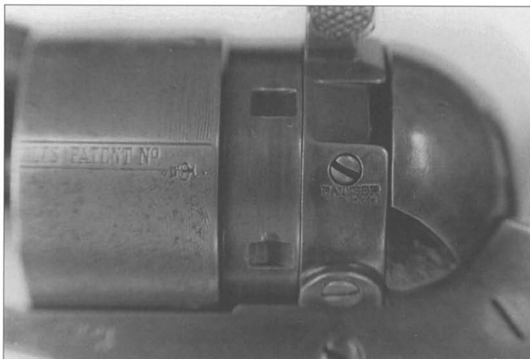
Fig. 4-74 Unnumbered Thuer conversion cylinder and patent date on conversion ring of 1860 Army Thuer conversion, serial number 95123. (Courtesy Francis E. "Bud" Firth)
