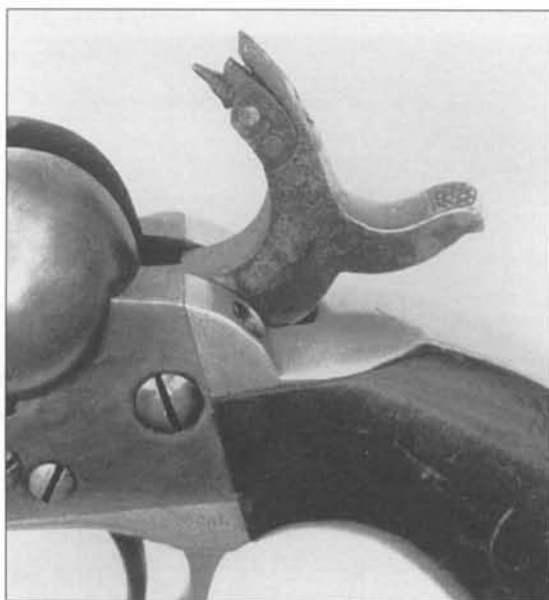
Fig. 8-66 Hammer of Colt Pocket Navy cartridge revolver, serial number 626, showing both firing pins.
