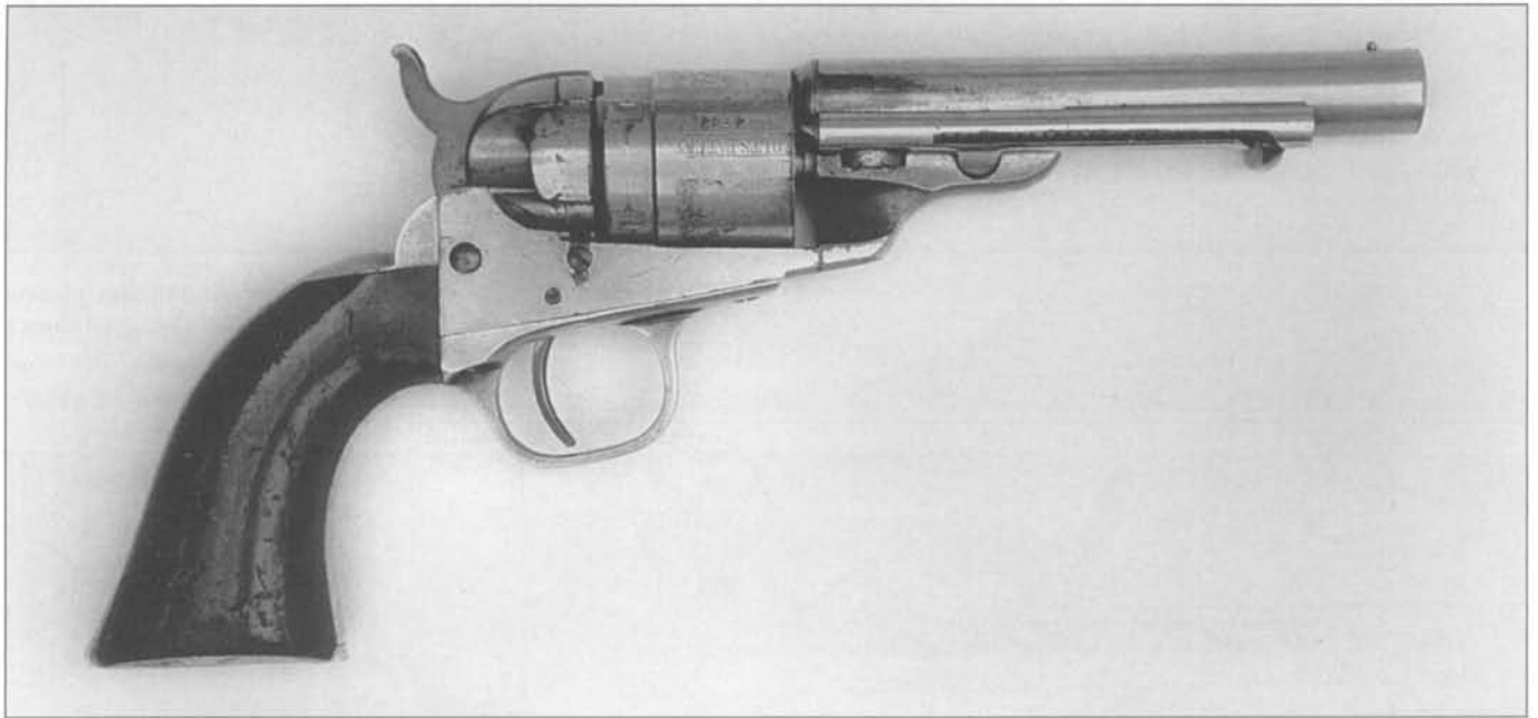
Fig. 8-71 Right side view of nickel-plated 4-1/2-inch Turned Round Barrel Colt Pocket Navy conversion, serial number 12932, assembly number 3896. (Author's Collection)
