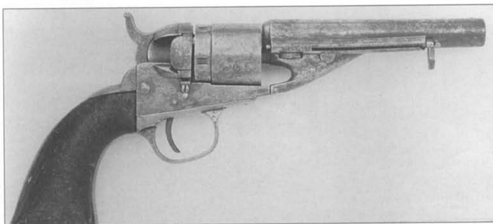
Fig. 8-39 Late production Colt Model 1862 Police cartridge revolver with external gate spring and large hammer screw. (Author's Collection)
