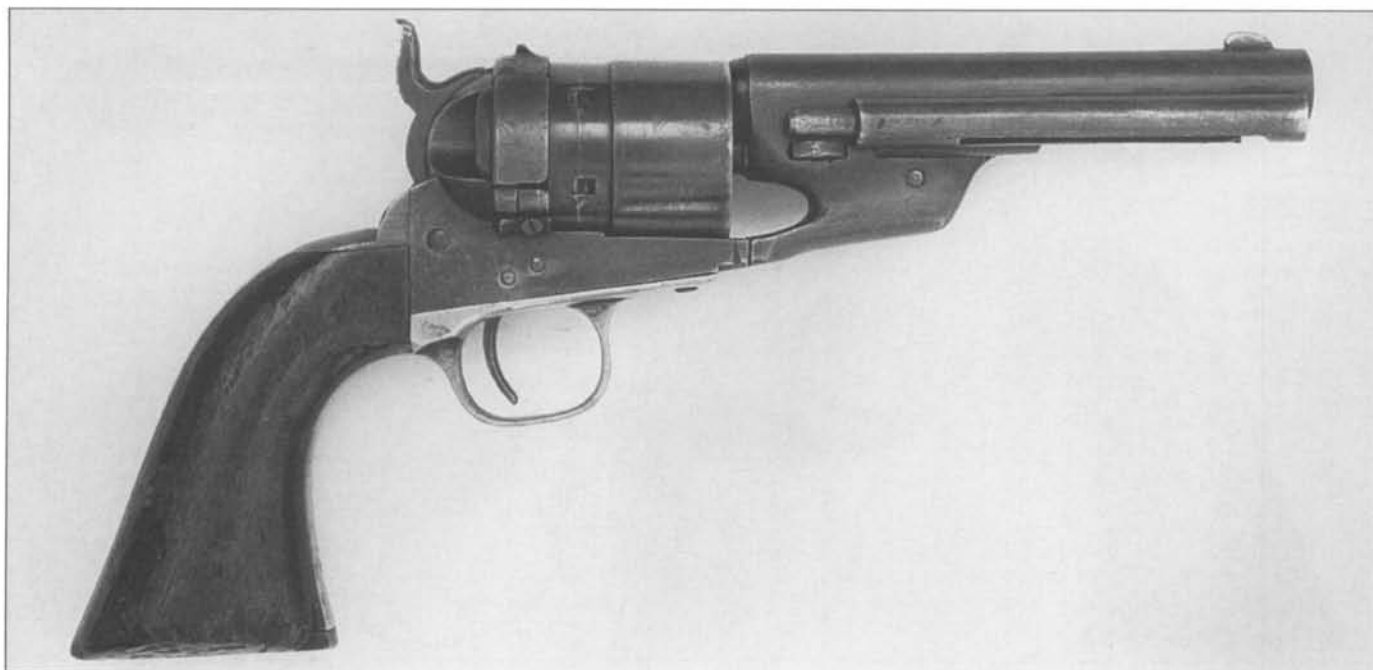
Fig. 9-37 Colt Model 1860 Richards conversion, serial number 2191, with barrel privately cut to 5-1/8 inches. (Author's Collection)
