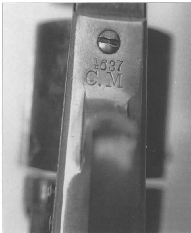
Above: Fig. 6-118 Underside of barrel of U.S. Navy Model 1861 Richards-Mason conversion with New York Navy Yard conversion inspector's stamp. Frame serial number 6957.
