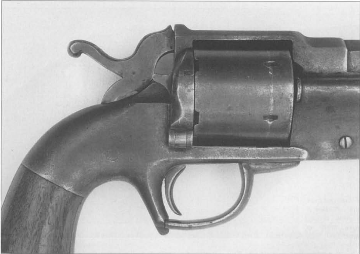
Fig. 10-47 Frame, cylinder, gate and hammer details of Allen & Wheelock Army Conversion, serial number 175.
