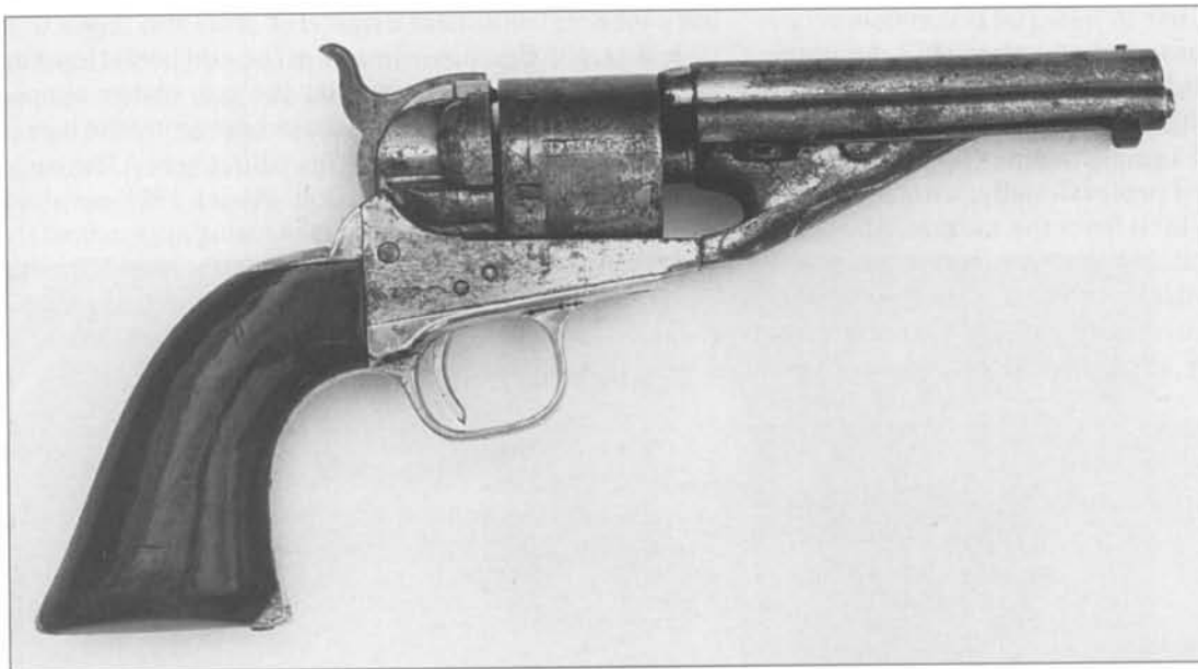
Fig. 9-43 Colt Model 1861 Navy conversion, serial number 743/1, with barrel privately cut to 4-3/8-inches. (Author's Collection)
