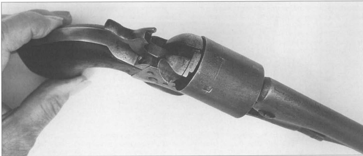
Fig. 9-54 Close-up of Model 1860 long cylinder frame, hammer face, hammer-stop and cylinder (top view). Serial number 10348. (Courtesy Francis E. "Bud" Firth)
