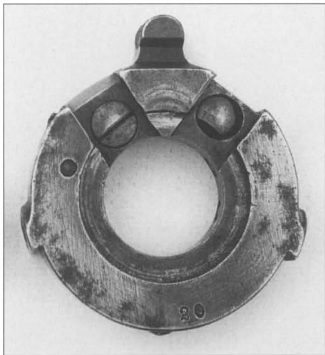
Fig. 4-22 Rear face of large frame conversion ring showing discharge and ejection pins, and conversion number 20.
