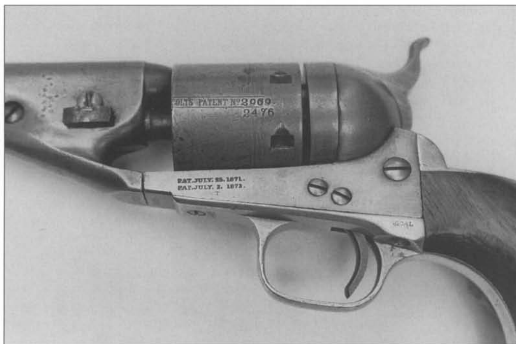
Fig. 6-124 Close-up of frame, barrel lug, cylinder and conversion ring of Model 1861 Navy-Navy conversion, serial number 2476, showing double cylinder number and frame stamping.
