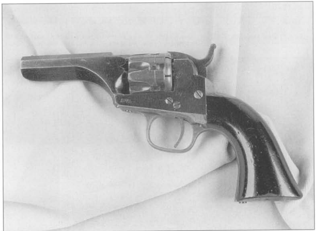
Fig. 9-1 An experimental Colt pocket revolver with two-piece cylinder. Serial number 226983. (Courtesy Francis E. "Bud" Firth)
