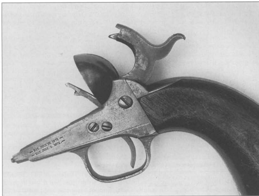
Fig. 6-62 Frame, hammer and hand close-up from percussion range Model 1851 Navy Richards-Mason conversion. (Author's Collection)
