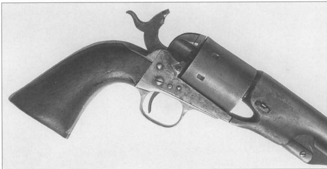
Fig. 9-53 Close-up of Model 1860 long cylinder frame, cartridge channel, hammer, firing pin, hammer-stop and cylinder (side view). Serial number 10348. (Courtesy Francis E. "Bud" Firth)
