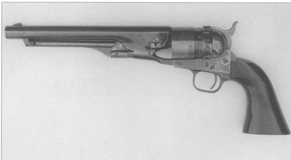
Fig. 4-63 Colt Model 1860 Army Thuer conversion with iron grip-strings and British proofs. Serial number 15453/L. (Courtesy John F. Dussling)
