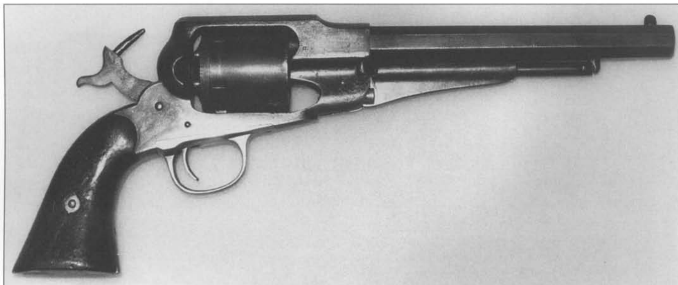
Fig. 3-44 Experimental Remington New Model Army converted for .44 caliber Martin centerfire cartridge. Serial number 109946. (Courtesy F. "Jay" Huber Jr.)
