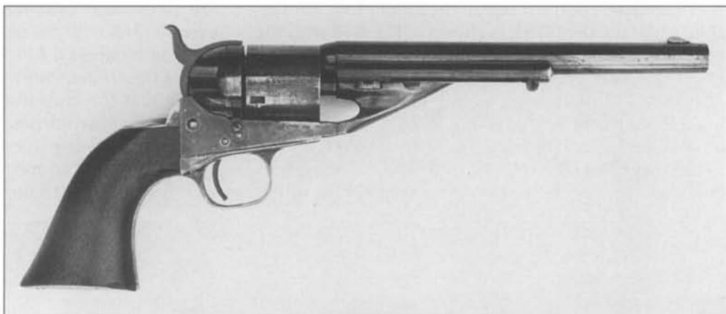
Fig. 6-100 Colt Model 1861 Percussion Range Richards-Mason conversion, serial number 31314, assembly number 1314, with British-proofed cylinder. (Courtesy John H. Thillmann)
