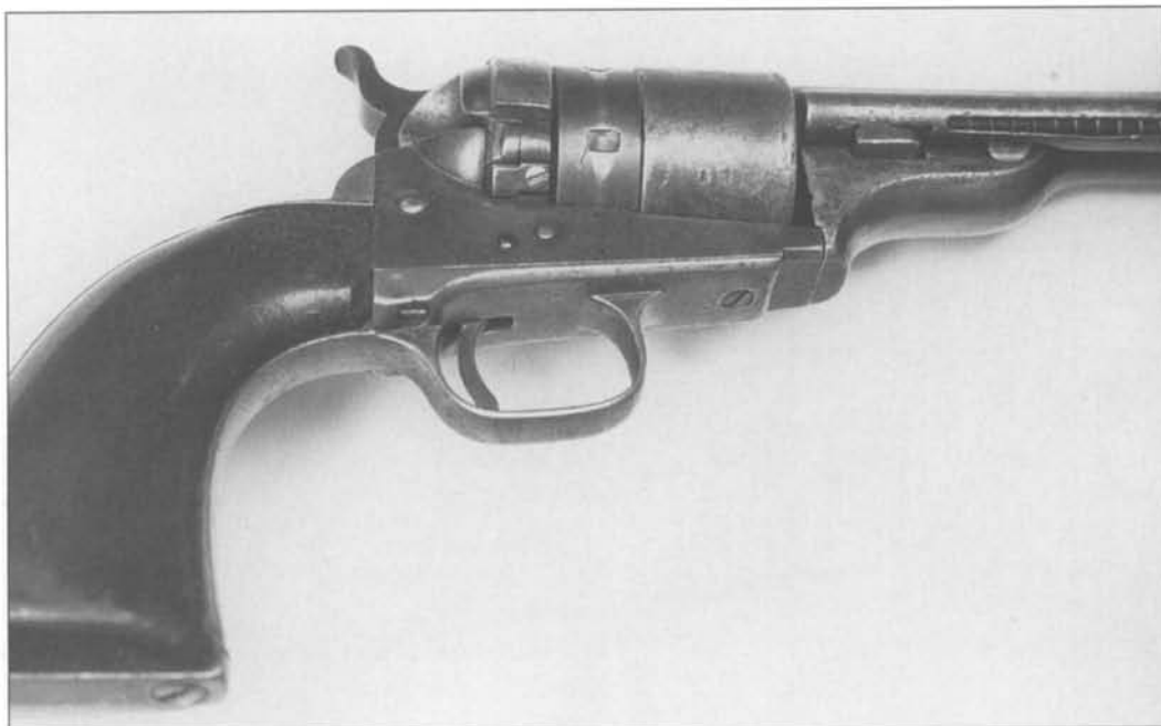
Fig. 6-9 Colt Model 1860 standard Richards-Mason conversion with civilian frame that has no shoulder stock cut-outs at recoil shield. (Author's Collection)
