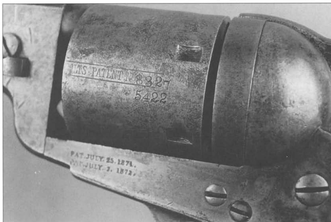
Fig. 6-68 Close-up of frame, barrel lug, cylinder and conversion ring of out of range Colt Model 1851 Navy-Navy conversion, showing two-line patent dates and dual cylinder numbering. Serial number 45422. (Courtesy Francis E. "Bud" Firth)
