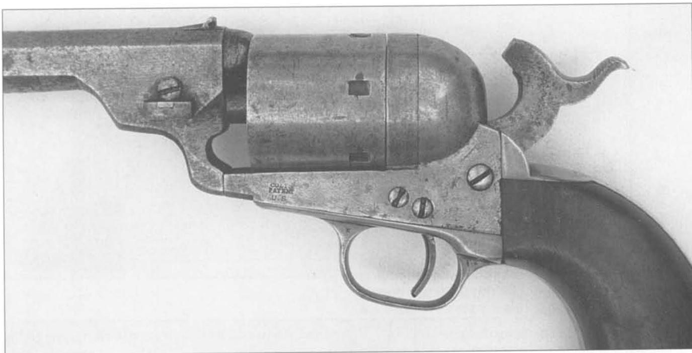
Fig. 9-19 Close-up of frame, conversion ring, cylinder and hammer of converted 1851 Navy revolver, serial number 57237. (Author's Collection)
