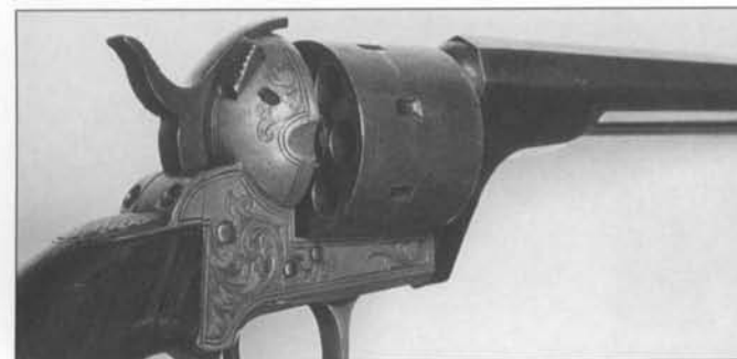
Fig. 1-18 Moore's rimfire revolver with barrel and cylinder rotated to right for loading.
