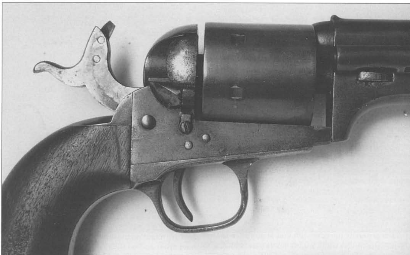
Fig. 7-11 Typical rimfire Model 1871-1872 Open Top revolver hammer, firing pin, frame, gate, gate spring, cylinder and breech cone of barrel.
