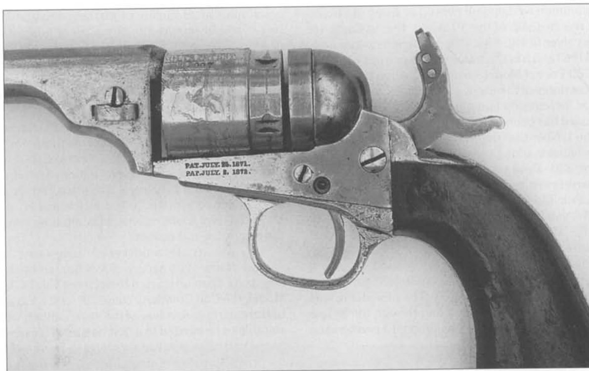
Fig. 8-89 Close-up of frame, cylinder and rimfire hammer of 3-1/2-inch Round Cartridge Barrel revolver, serial number 3007. (Author's Collection)
