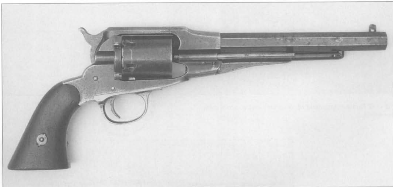
Fig. 3-81 Standard Remington New Model Navy revolver factory converted to .38 caliber rimfire. Serial number 44955. (Author's Collection)
