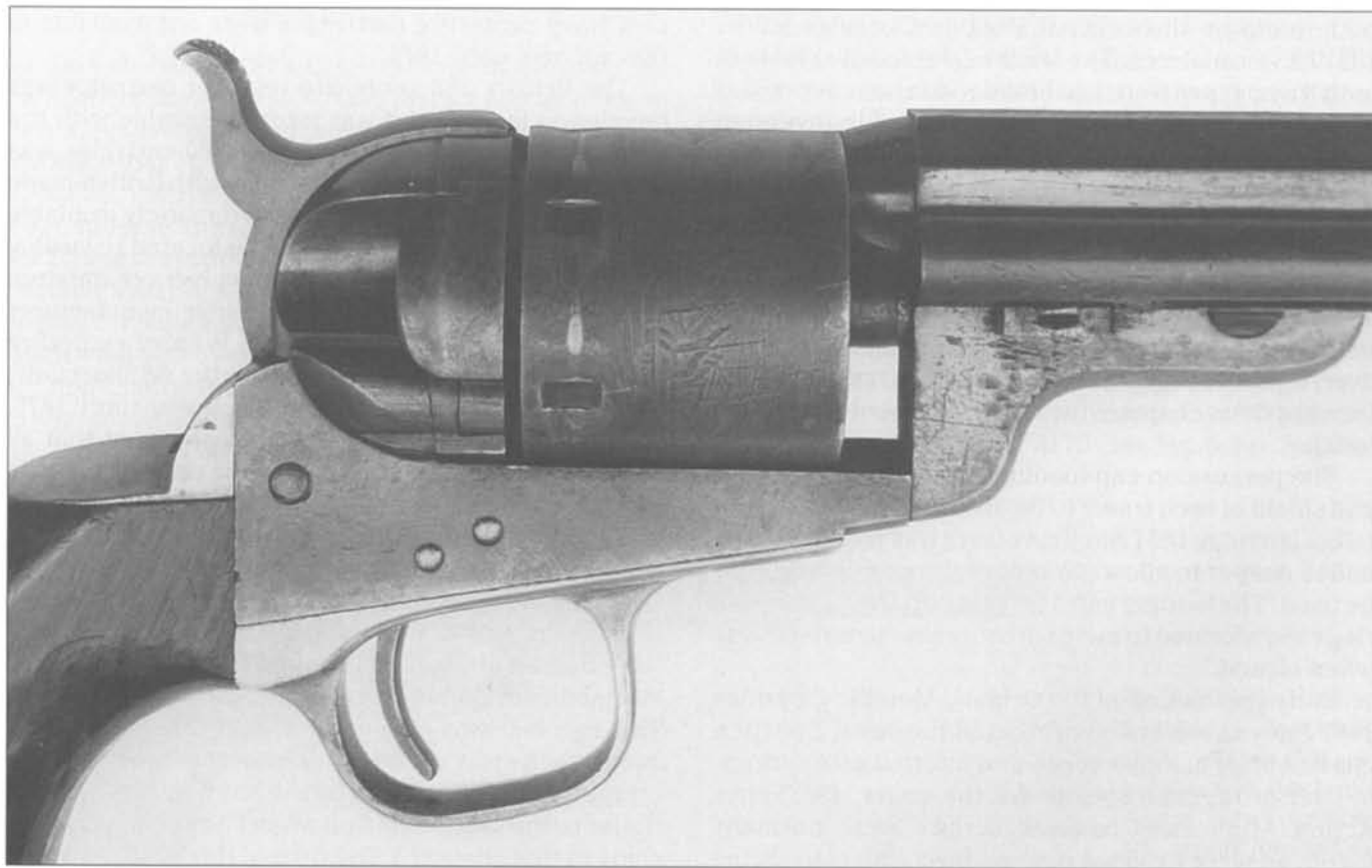
Fig. 6-47 Close-up of Model 1851 Richards-Mason frame, cylinder and barrel lug, showing no loading cut-out at barrel lug. Serial number 437. (Courtesy Dow and Russelle Heard)
