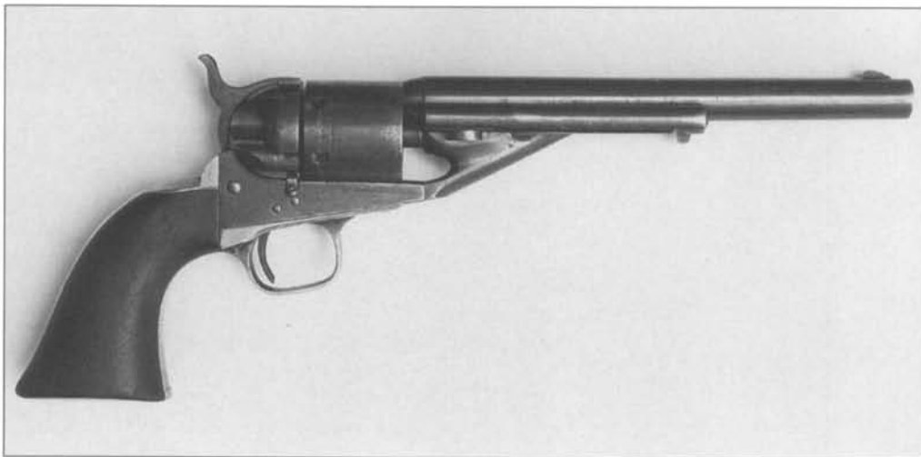
Fig. 6-116 Right side of mixed number U.S. Navy Model 1861 Richards-Mason conversion showing external gate spring and deepened loading channel. (Author's Collection)
