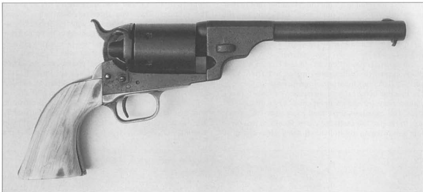
Fig. 9-30 Right side of Colt Third Model Dragoon conversion, serial number 11907. (Author's Collection)
