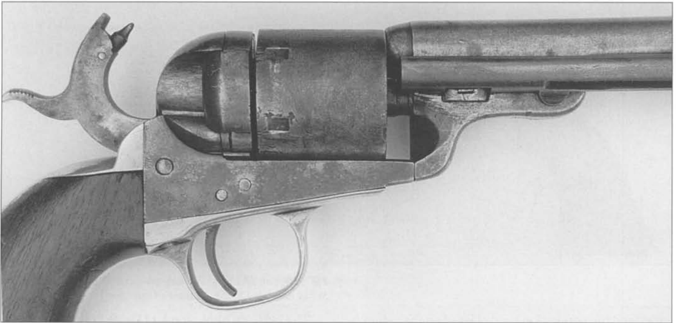
Fig. 9-26 Firing pin, loading gate and ejector housing detail of round barrel 1851 Navy conversion. Serial number 130858. (Author's Collection)
