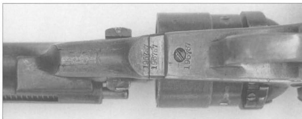
Fig. 5-84 Second Model Richards, serial number 196787; left side close-up of frame, hammer, cylinder and conversion ring.
