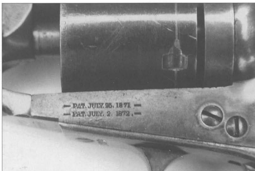
Fig. 6-41 Two-line patent dates on Original Metallic Cartridge Colt Model 1861 Navy conversion, period at end of top line missing because of broken die. (Courtesy Francis R. "Bud" Firth)
