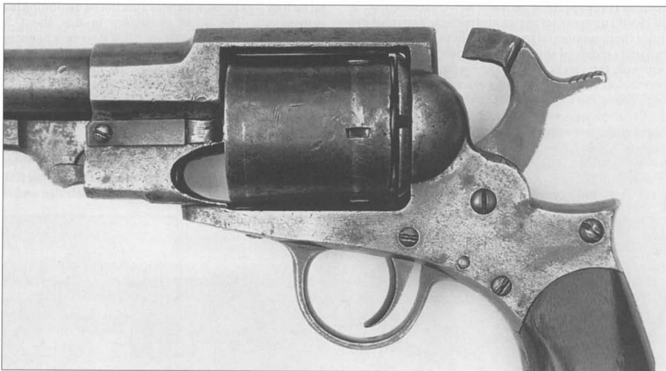
Fig. 10-22 Left side view of frame, cylinder, hammer, backing plate and thumbcatch spring of the Austin T. Freeman conversion.
