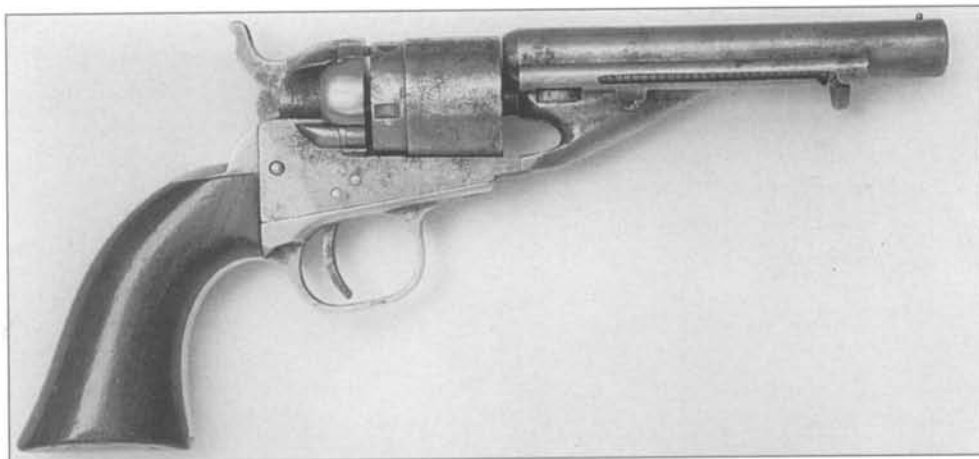
Fig. 8-38 Early production Colt Model 1862 Police cartridge revolver with internal gate spring and small hammer screw. (Author's Collection)
