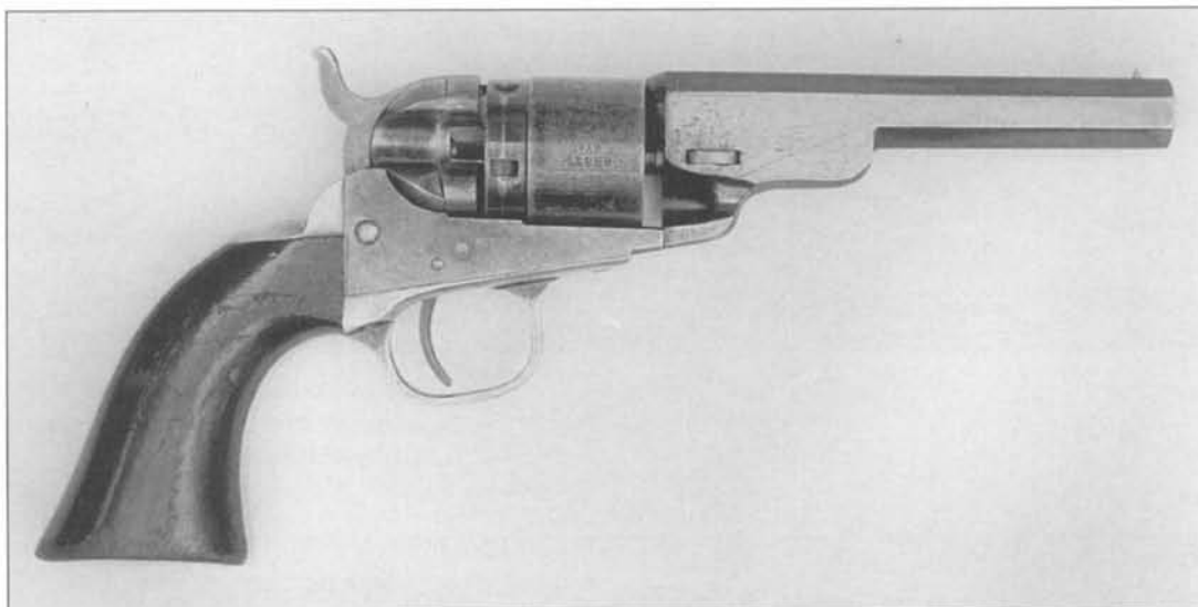
Fig. 8-57 Right side view of 4-1/2-inch Colt Pocket Navy conversion, made without loading gate and double-numbered cylinder. Serial number 18765. (Author's Collection)
