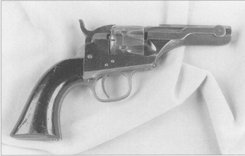
Fig. 9-2 The sliding cartridge extractor rod of experimental Colt. Serial number 226983. (Courtesy Francis E. "Bud" Firth)
