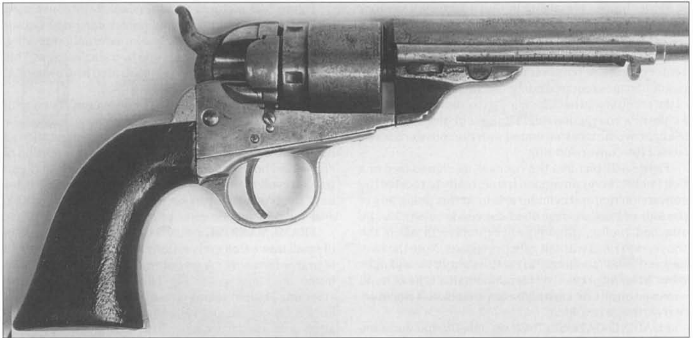
Fig. 8-23 Typical Turned Round Barrel Colt Pocket Navy conversion with a round rebated cylinder and an external gate spring.
