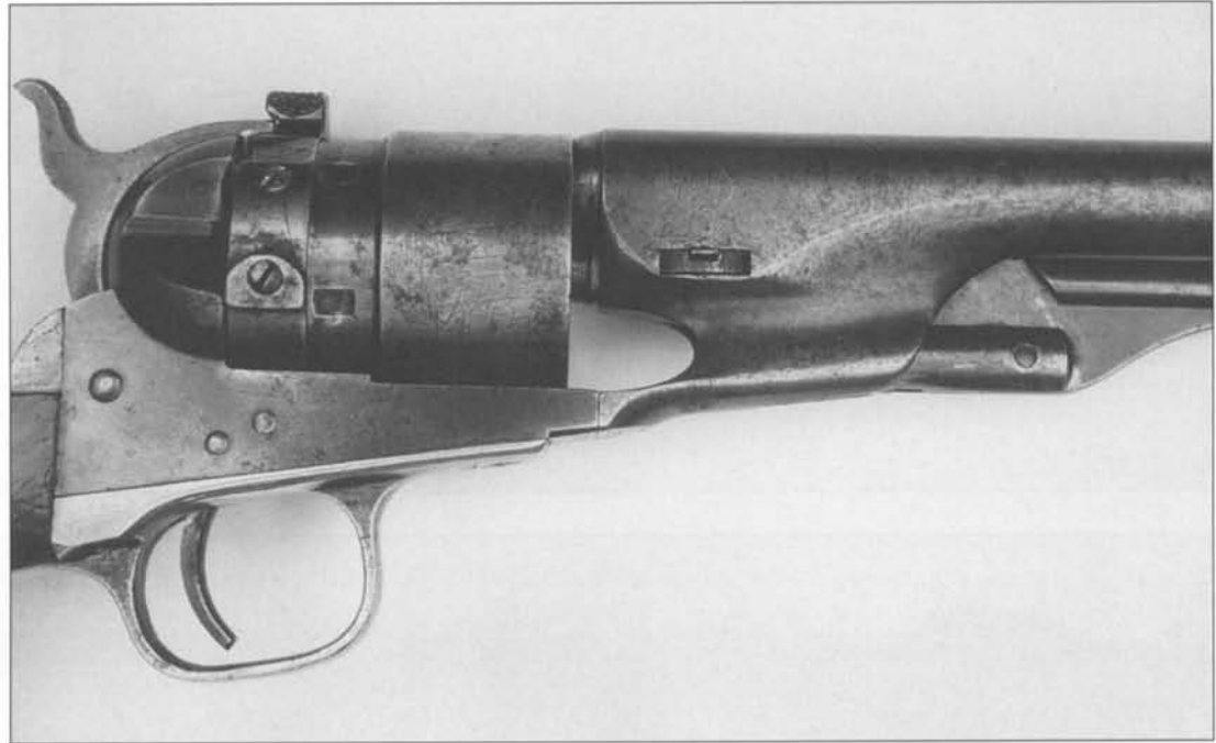
Fig. 4-4 Scooped out barrel lug loading channel of Hartford Colt Model 1860 Army Thuer conversion.
