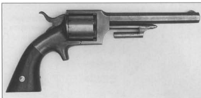
Fig. 2-26 Pond front loading revolver with chamber tubes and final ejection stem. Six shots, .32 caliber, serial number 899. (Author's Collection)
