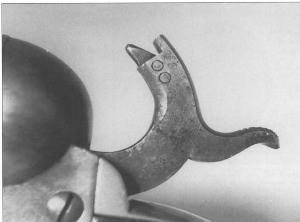
Fig. 6-34 A Richards-Mason 1860 Army Hammer fitted to an 1851 Navy-Navy conversion, serial number 59721. (Photo by L. Frank Richey, Sam Pachanian Collection)
