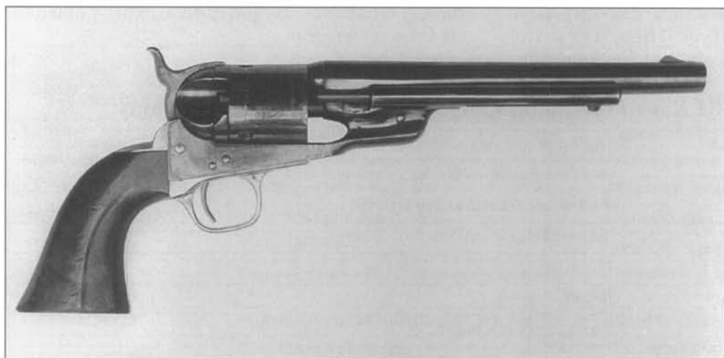
Fig. 6-92 Factory experimental Model 1861 Richards-Mason conversion. Right side view shows Richards-type ejector system and the Type III Richards-Mason conversion ring. No loading gate is incorporated. (Courtesy Francis E. "Bud" Firth)
