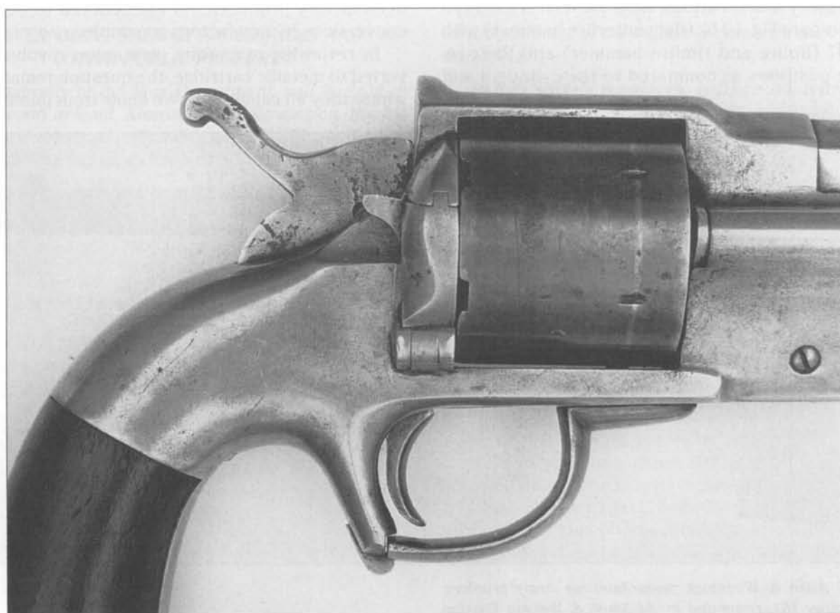
Fig. 10-52 Altered hammer position of Allen & Wheelock Army centerfire conversion, serial number 96.
