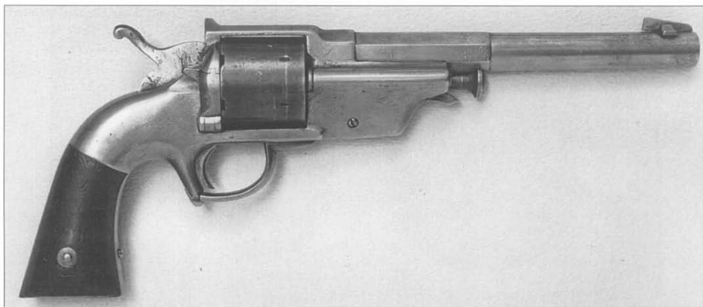
Fig. 10-50 Allen & Wheelock center hammer Army revolver, serial number 96, converted to centerfire S&W Russian cartridge. (Author's Collection)
