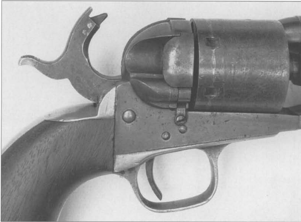
Fig. 6-88 Less common blade-type centerfire firing pin found mounted within slot cut at center of Model 1861 hammers and maintained by two rivets.
