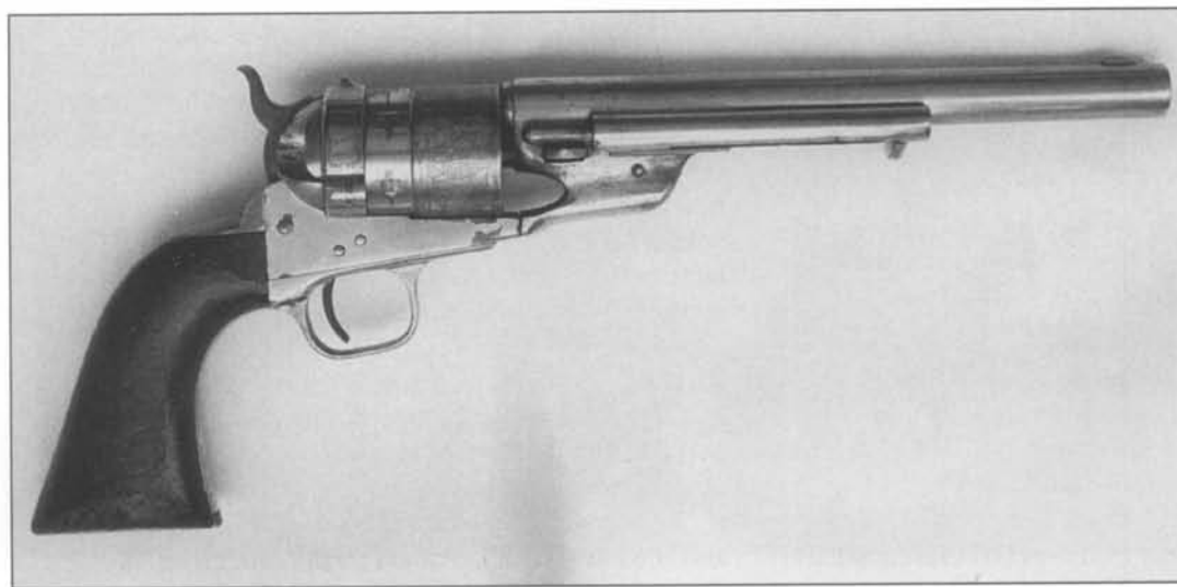
Fig. 5-40 First Model Richards conversion Model Gun, assembly number 1131 and stamped "M". (Courtesy Francis E. "Bud" Firth)
