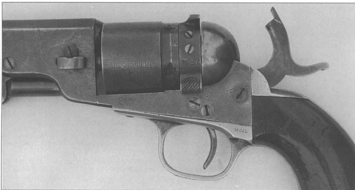
Fig. 4-50 Cylinder and conversion ring of Colt Pocket Navy showing ring in eject position.
