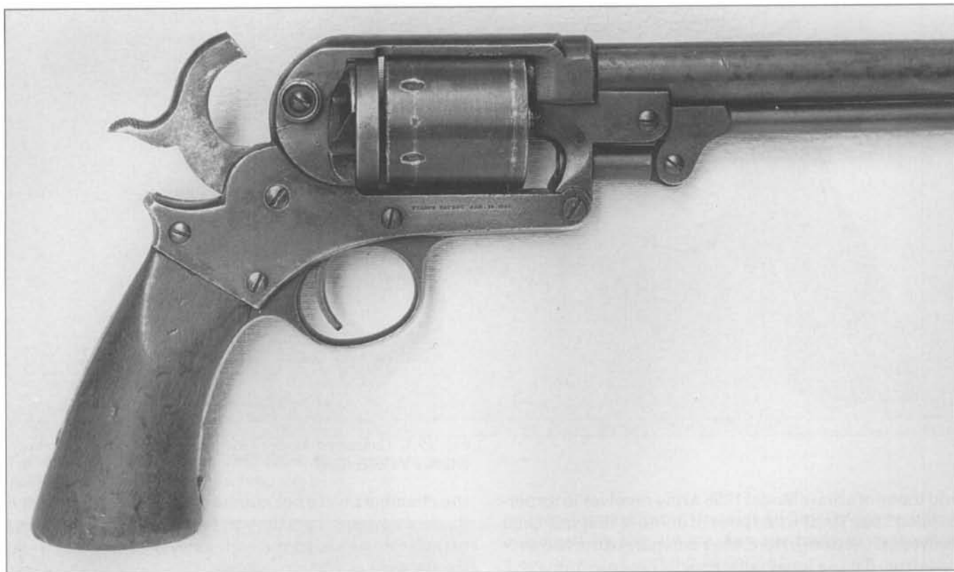
Fig. 10-38 Frame, conversion ring, cylinder and hammer detail of Starr Model 1863 conversion.
