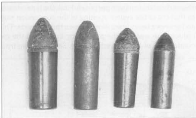
Fig. 4-7 Four basic sizes of Thuer metallic centerfire cartridges. Left to right: .44 Army, .36 Navy, .36 Pocket Navy and .31 Pocket. (Courtesy Francis E. "Bud" Firth)
