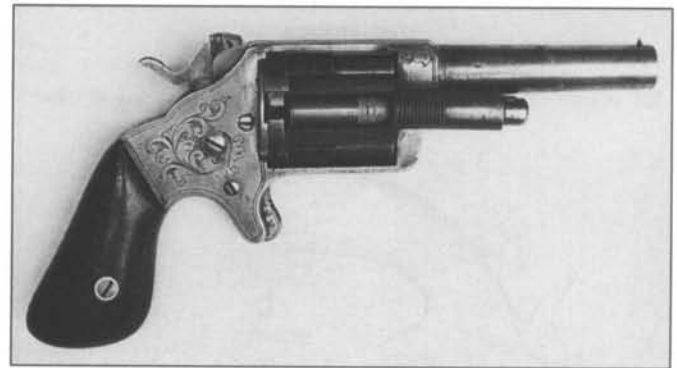
Fig. 2-29 Slocum revolver with a chamber tube forward over the ejector stem and fresh cartridge in cylinder.
