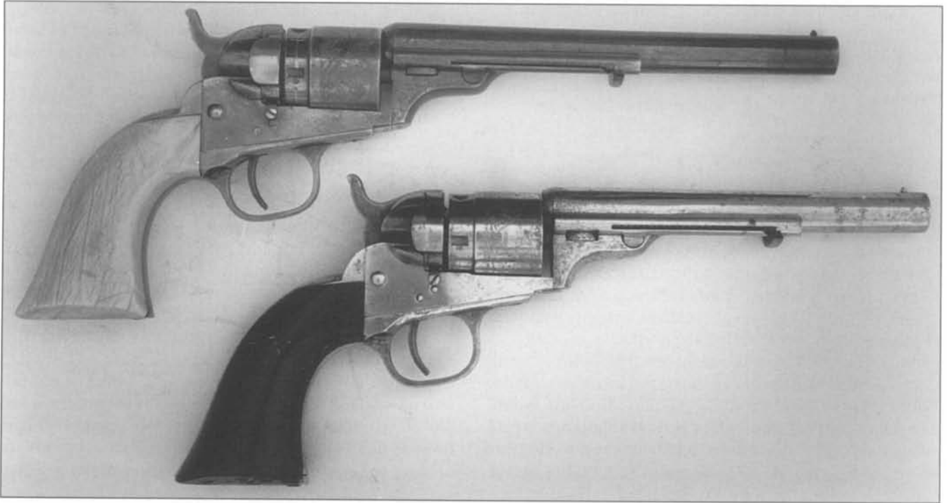
Fig. 8-93 Two Round "S" Lug Cartridge Barrel Pocket Navy conversions: (Top) Serial number 46833 with 6-1/2-inch barrel; (Bottom) Serial number 10559 with 5-1/2-inch barrel. (Courtesy John H. Thillmann)
