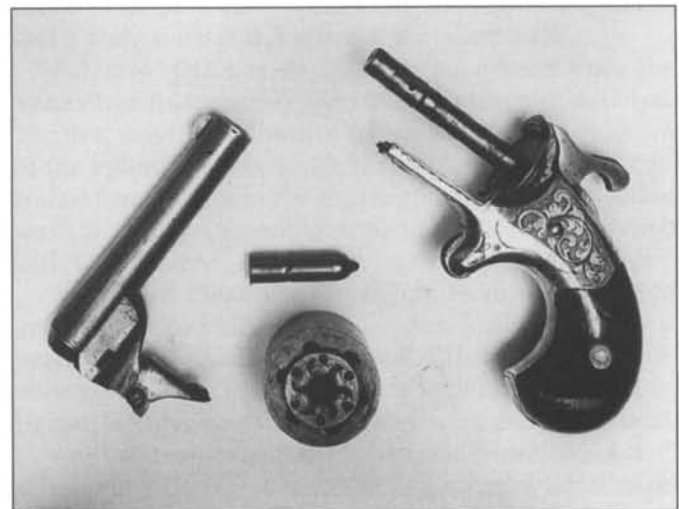
Fig. 2-12 Moore's teat-fire disassembled.
