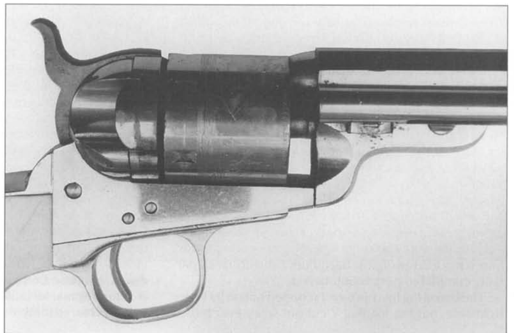
Fig. 6-45 Frame, cylinder and barrel lug close-up of Original Metallic Cartridge Richards-Mason revolver showing partially completed percussion barrel, scooped out at the lug but no "V" loading notch cut. (Courtesy Dow and Russelle Heard)
