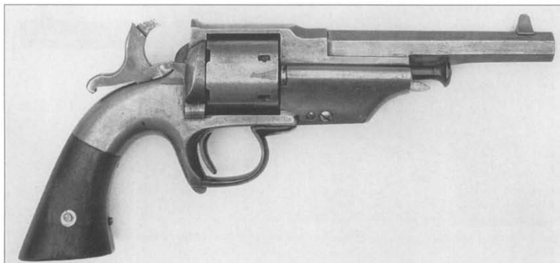
Fig. 10-44 Allen & Wheelock center-hammer Navy revolver, serial number 46, converted to rimfire cartridge. (Author's Collection)
