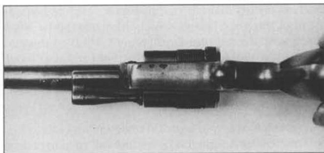
Fig. 2-32 Underside of Slocum revolver frame, showing the final cartridge ejector stem.
